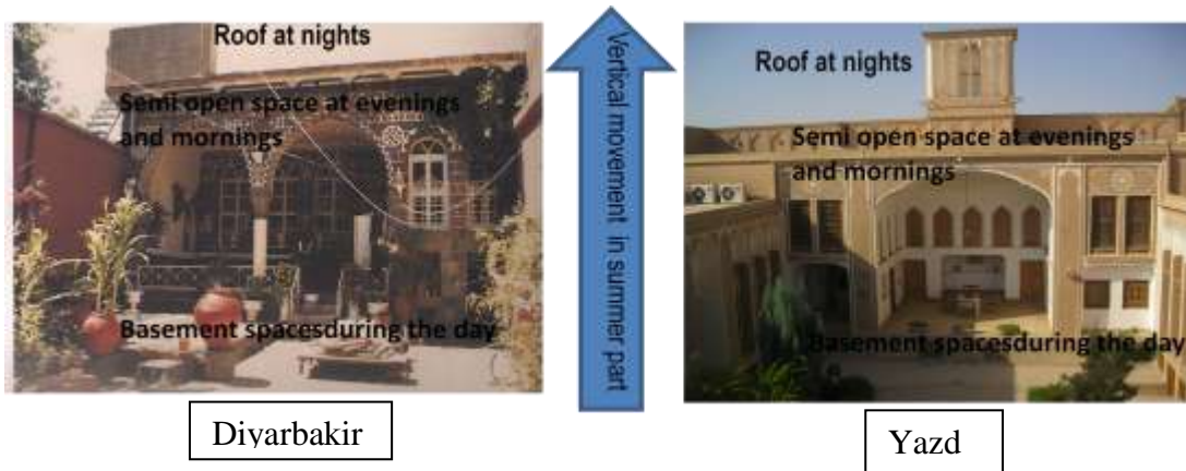
Figure 61: Vertical movement of inhabitant in summer parts of Diyarbakir and Yazd traditional houses (Tuncer,1999)
