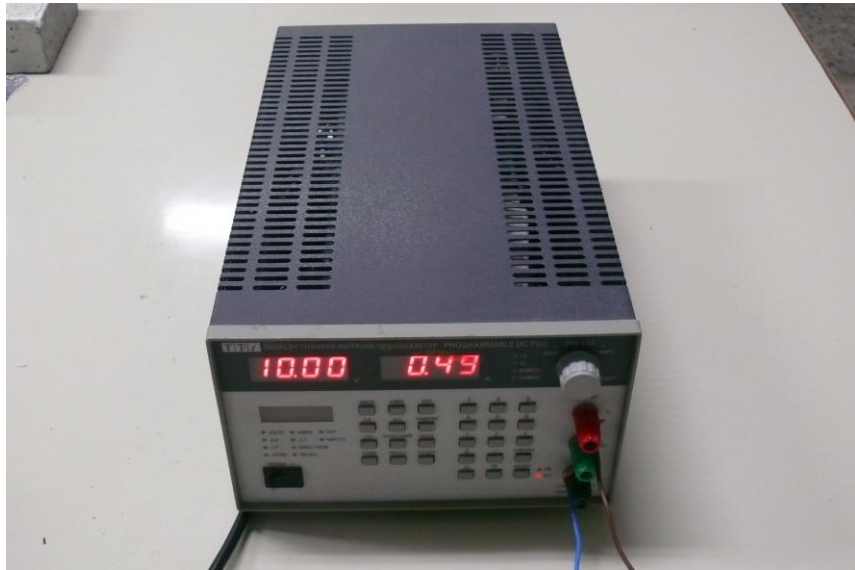
Figure 9: Variable voltage transformer (programmable DC PSU type TSX3510P-TTI).
