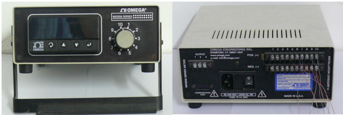
Figure 10: A ten channel data acquisition box from OMEGA series MDSSi8.
