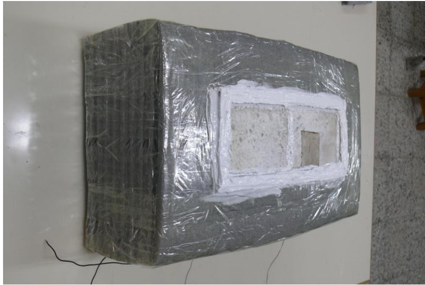
Figure 8: The specimen inserted, fitted, and well sealed (except one surface).
