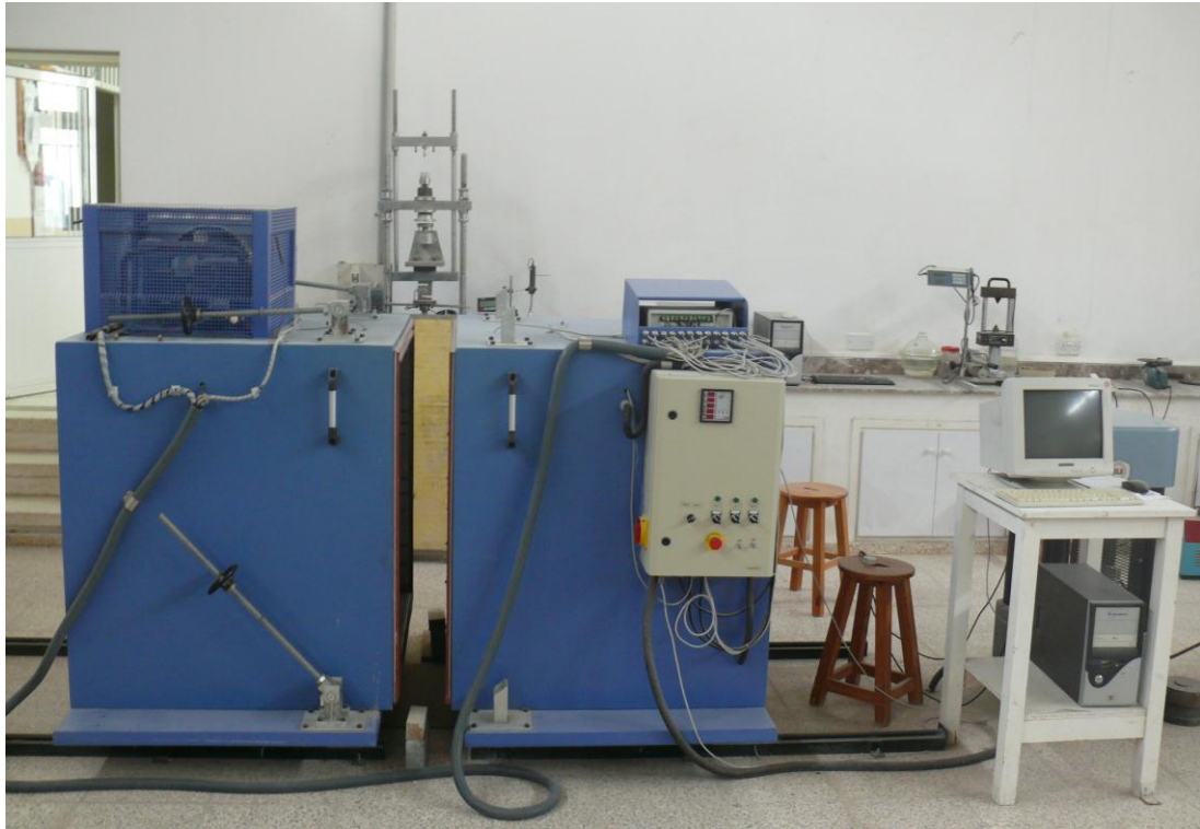
Figure 4: Hot Box apparatus available in the Civil Engineering Department at the EMU
