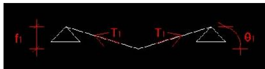
Figure 2.4 The cable then undergoes a deflection.
