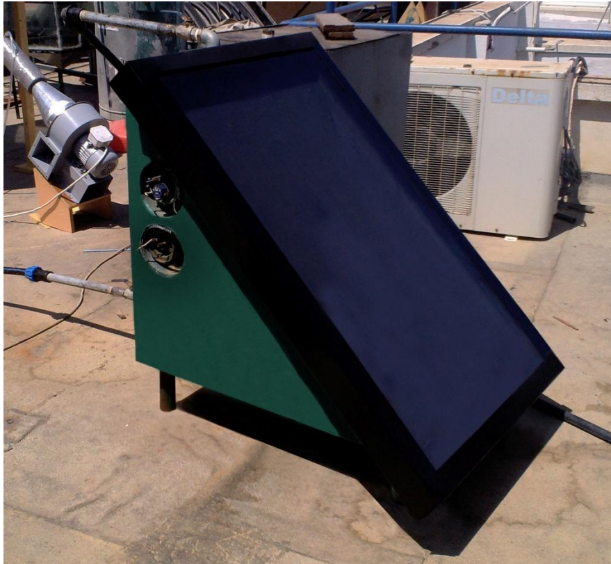
Figure 2.3. The new integrated solar water heater.
