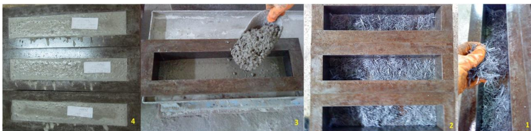
Figure 1 - Placement of fibers for SIFCON
