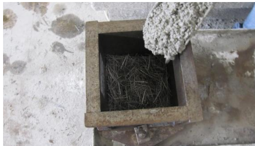
Figure 16 - Filling molds with mortar
