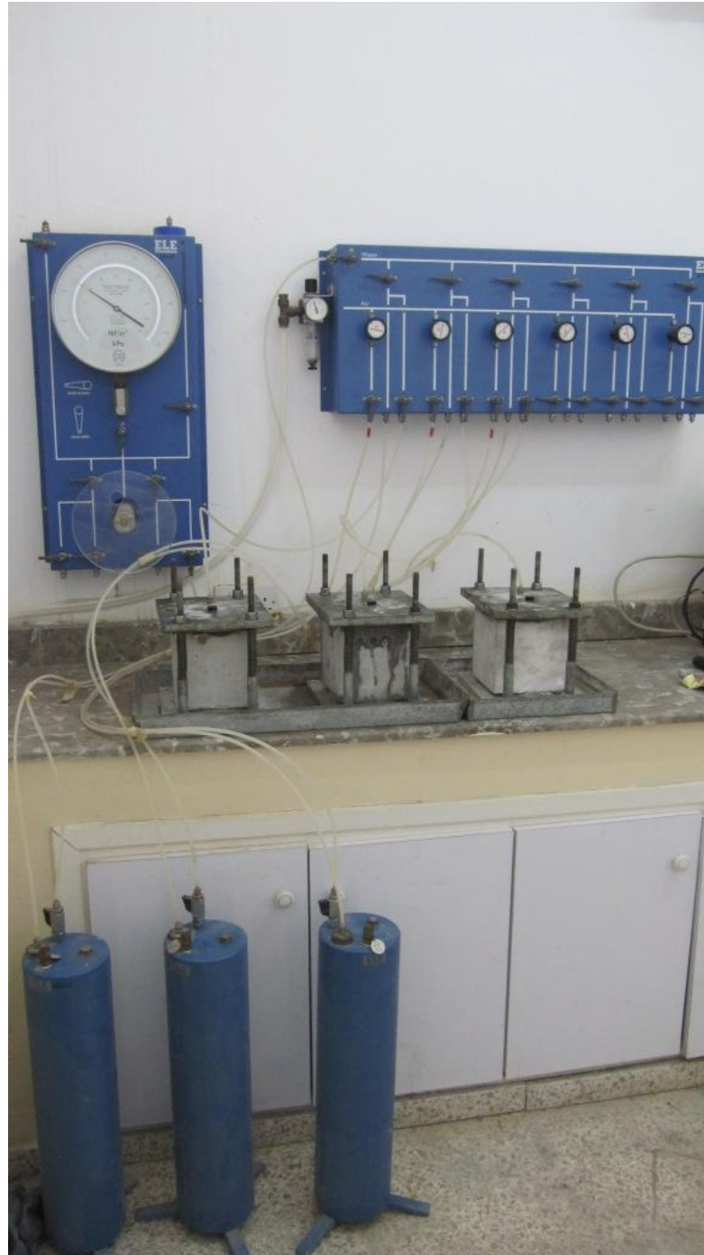
Figure 23 - Apparatus for water permeability test
