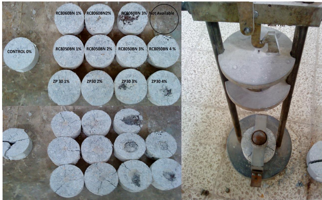
Figure 21- Specimens before and after test energy Impact test
