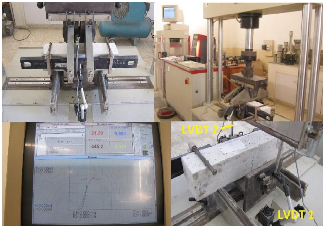
Figure 18 - Flexural third point test apparatus
