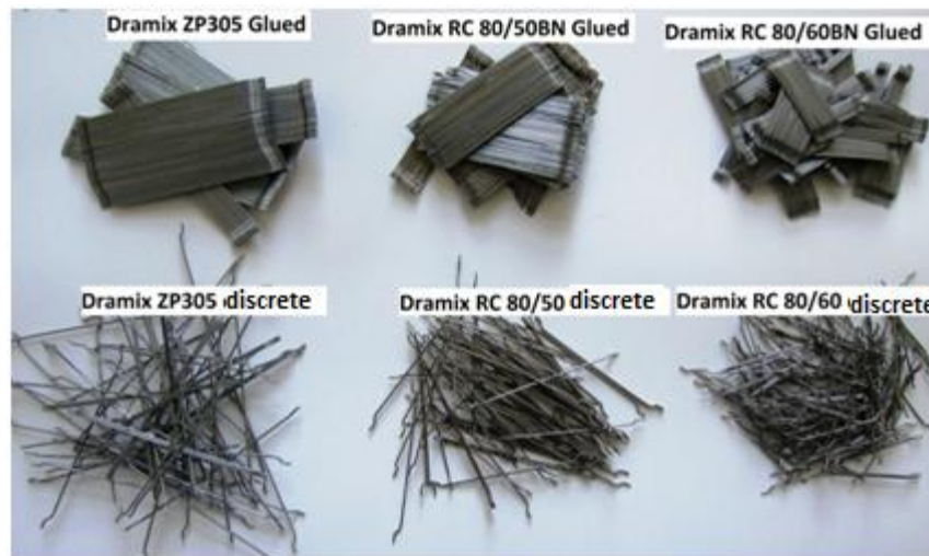
Figure 15 - Fibre types used in this study
