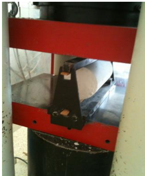
Figure 3.11: Cylinder specimen under splitting tension
