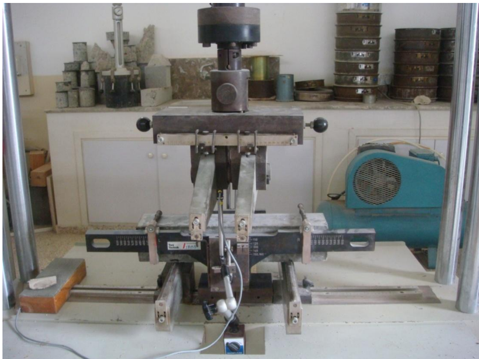
Figure 3.9: Beam specimen under flexural strength
