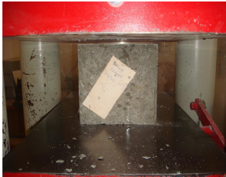
Figure 3.7: Cubic sample under compression in the machine
