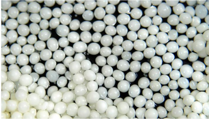
Figure A-3.1.4. Chitin-g-P4VP Beads after the Soxhlet Purification in Et-OH, before Water Purified.
