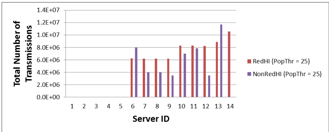
Figure 7.15: Server ID versus Total Number of Transmissions for RED-Hi and Pure Hierarchy with arrival rate 0.2 and Popularity Threshold of 25.
