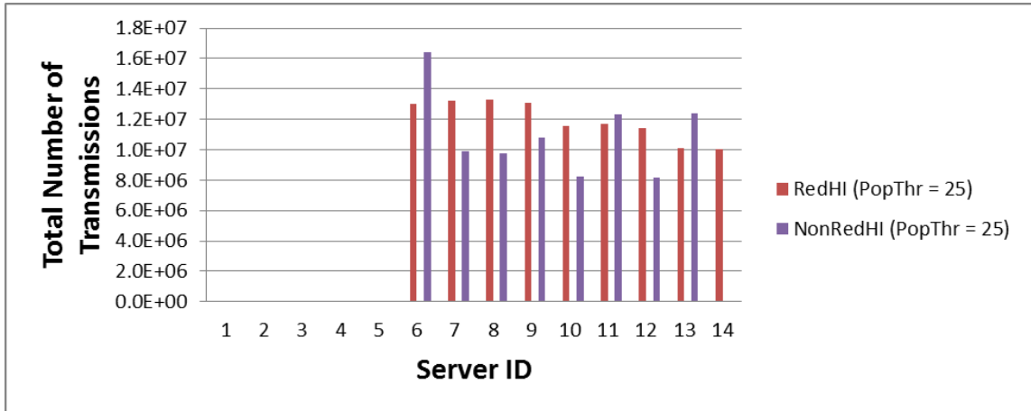
Figure 7.12: Server ID versus Total Number of Transmissions for RED-Hi and Pure Hierarchy with arrival rate 0.05 and Popularity Threshold of 25.
