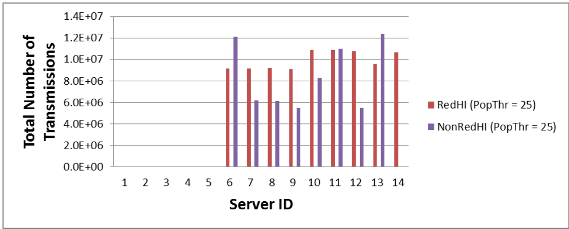
Figure 7.14: Server ID versus Total Number of Transmissions for RED-Hi and Pure Hierarchy with arrival rate 0.15 and Popularity Threshold of 25.
