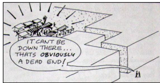
Figure 3.15: In spite of being physical permeable, there is no visual permeability (Bentley, 1985)
