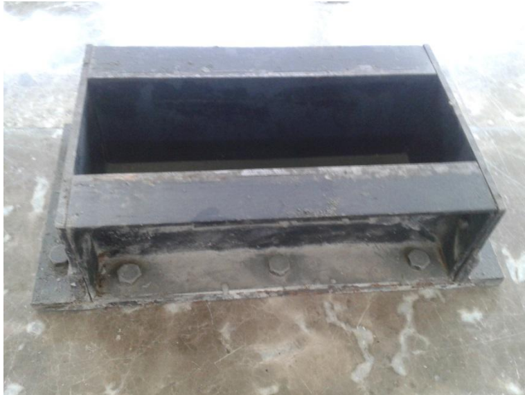
Figure4. Steel molds for beams
