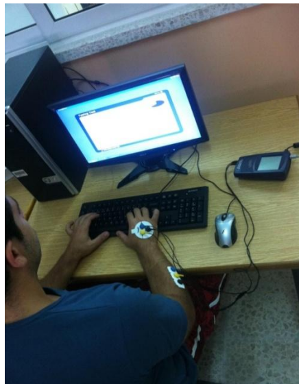
Figure 3: Placement of sEMG Electrodes on Wrist (flexor retinaculum) and Elbow (extensor digitorum)
