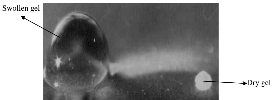
Figure 1: Schematic illustration of SAHs swelling with Comparison of the dry and swollen state particle
