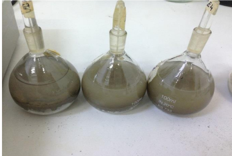
Figure 3.4: Specific gravity test on soil sample and stabilizers
