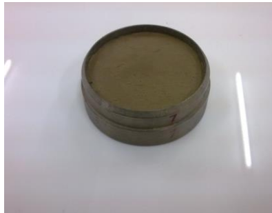
Figure 3.14: Sample in the metal ring (50 mm diameter and 20 mm height)
