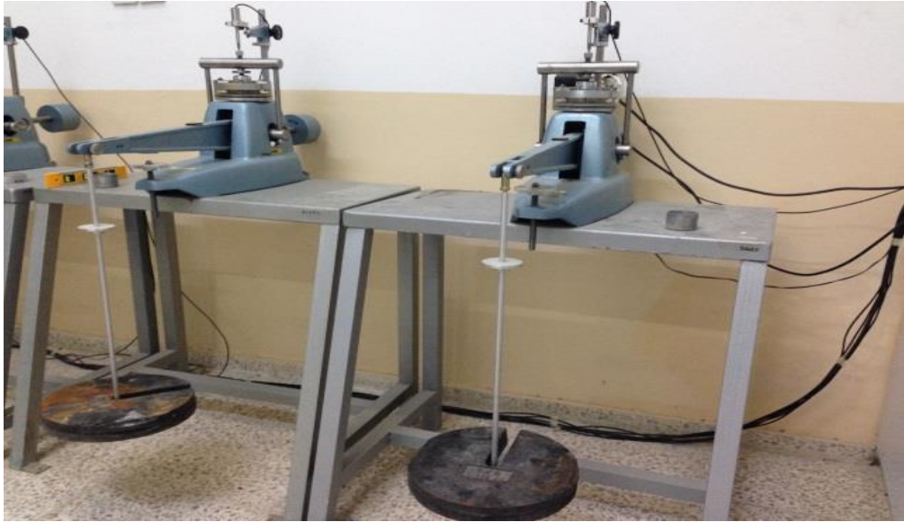
Figure 3.19: Consolidation test with the transducers connected to ADU system
