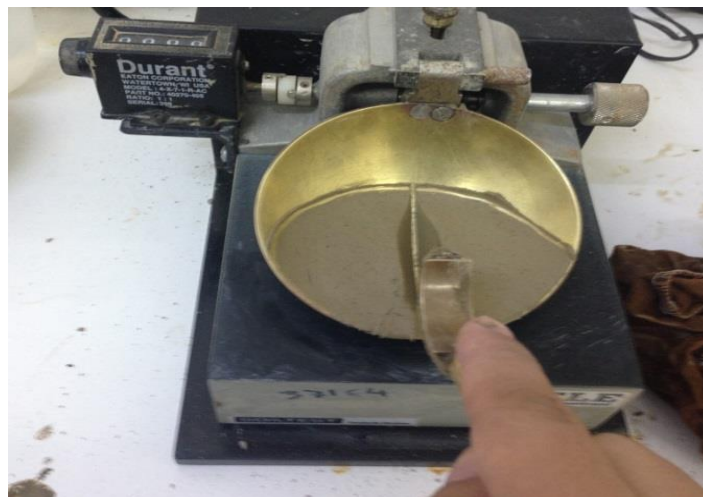
Figure 3.8: A groove was made in the middle of sample
