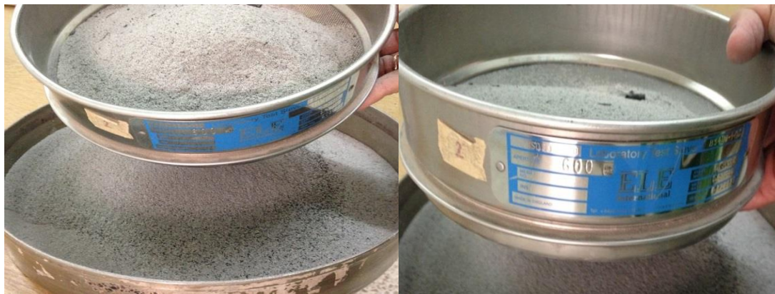
Figure 3.2: Sieving RHA through 600 µm sieve
