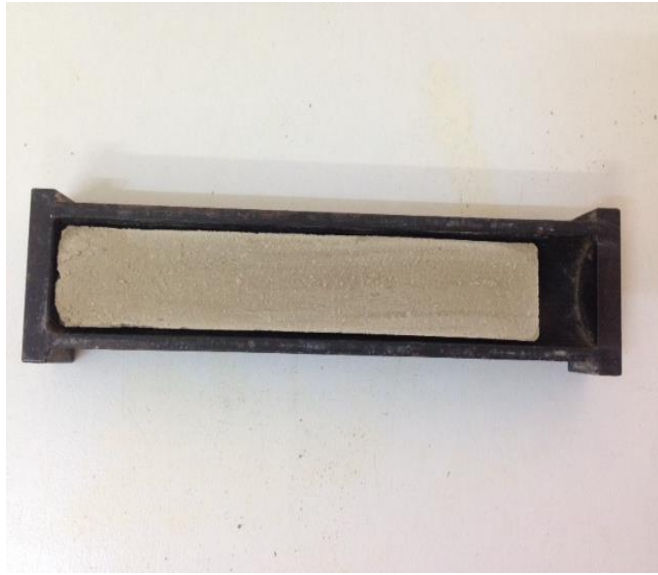
Figure 3.10: Reduction of length of sample in linear shrinkage mold
