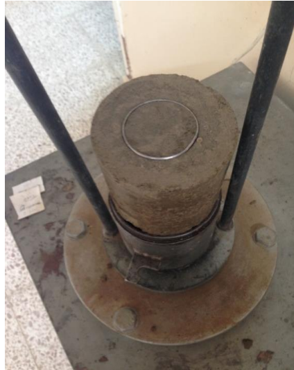
Figure 3.13: Recovering samples from the compaction mold
