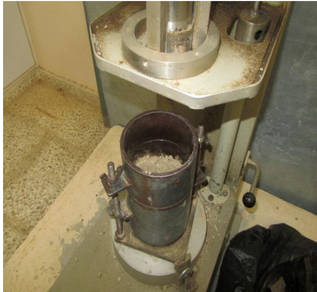
Figure 3.11: Standard compaction mold
