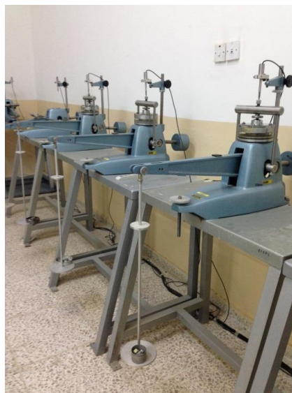
Figure 3.15: Samples in oedometer for one-dimensional swell-consolidation testing
