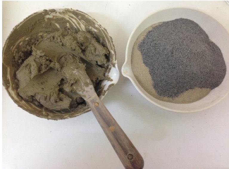
Figure 3.7: Soaking and mixing sample with distilled water
