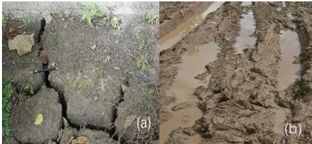
Figure 2.2: (a) Shrinkage and (b) swelling of expansive soil
