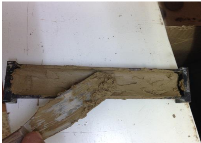
Figure 3.9: Rubbing the soil in linear shrinkage mold
