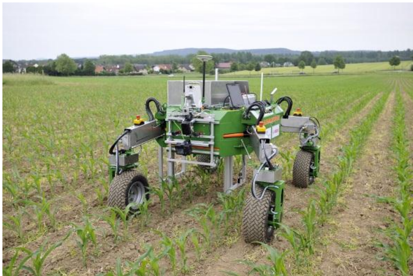
Figure 1: Agriculture Robot while recognizing the bad grass and weeds in the fields
