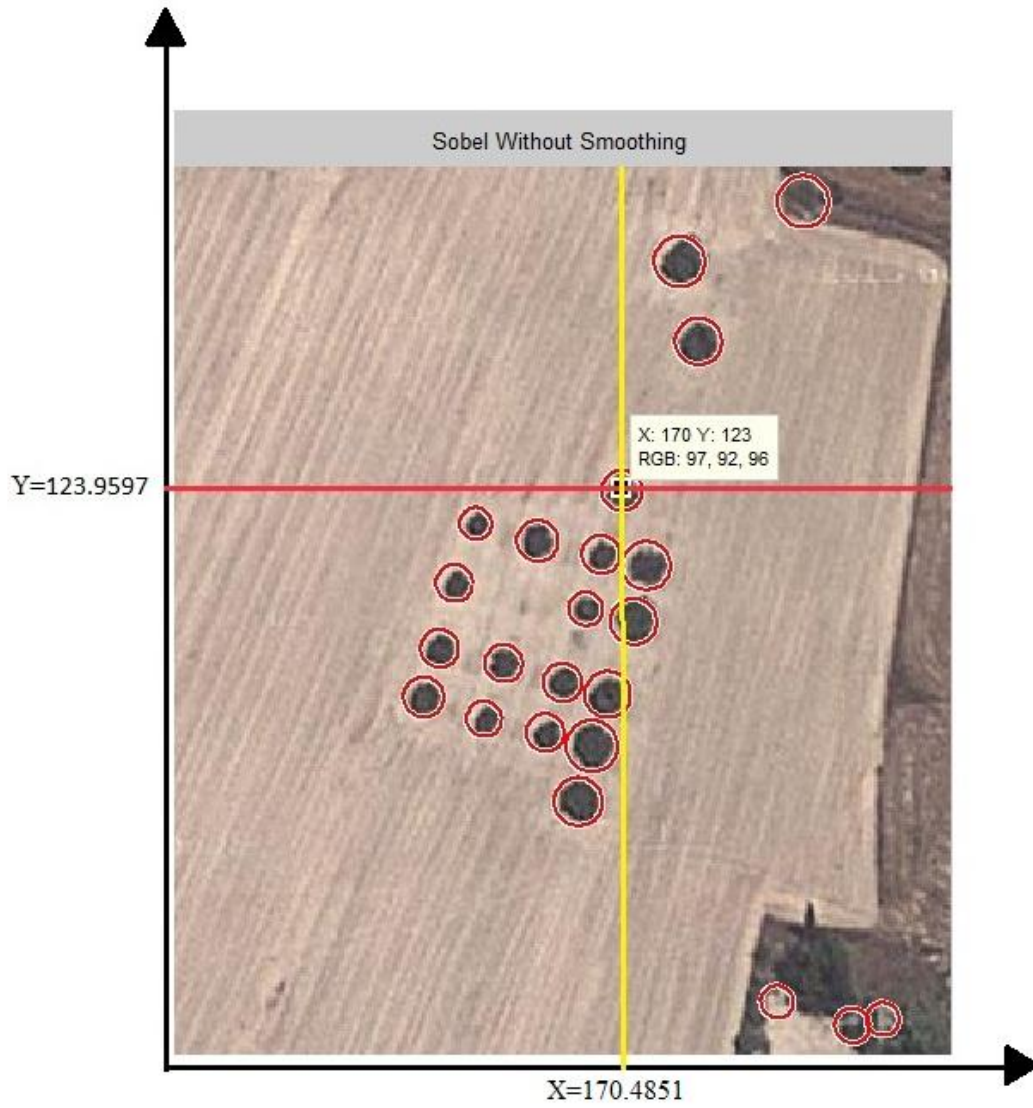
Figure 12: Mapping of field coordinates to the center pixel of obstacles in original image
