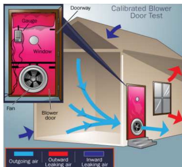
Figure 7: Blower door test (ISOVER, 2008)
