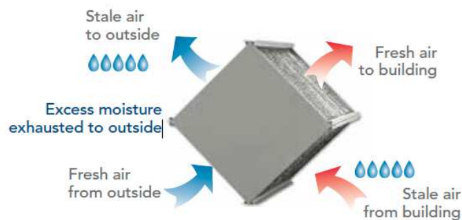
Figure 9: HRV (Heat Recovery Ventilator)
