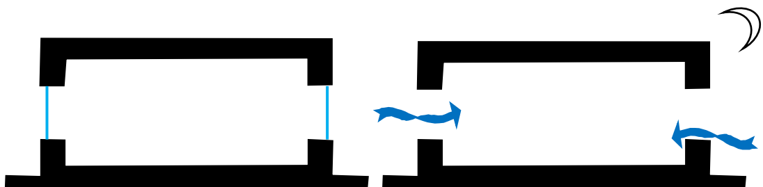
Figure 17: Left: Cooling with thermal mass; Right: Night cooling with high thermal mass (Brown, 2001)
