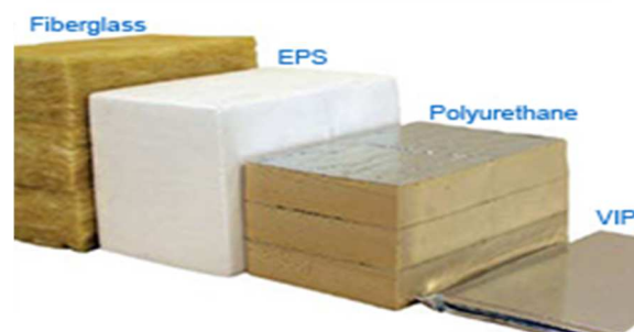
Figure 3: Thickness comparison between several insulation-materials. ( http://www.sealedairspecialtymaterials.com )
