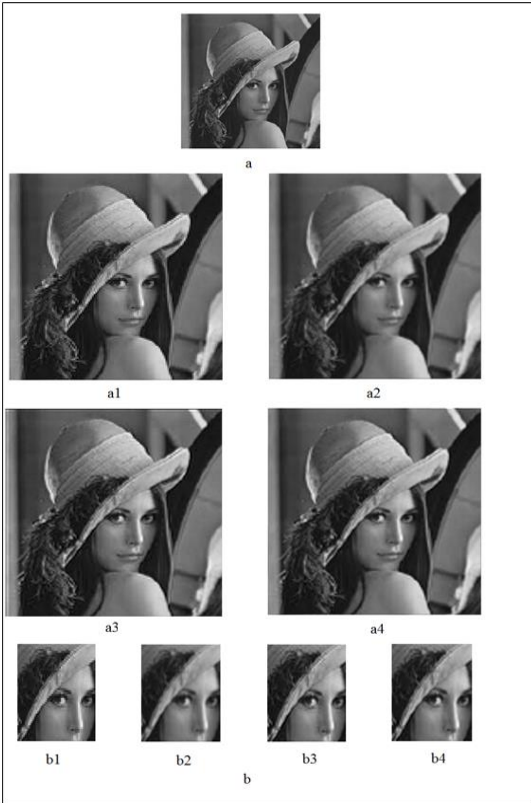
Figure 3.17: Scaled the Lena image by two: a1) nearest, a2) linear, a3) SLI, and a4) cubic interpolation, the sharpest image belongs to the SLI's image. b) Zoomed images b1, b2, b3 and b4 of a1, a2, a3, and a4, respectively.
