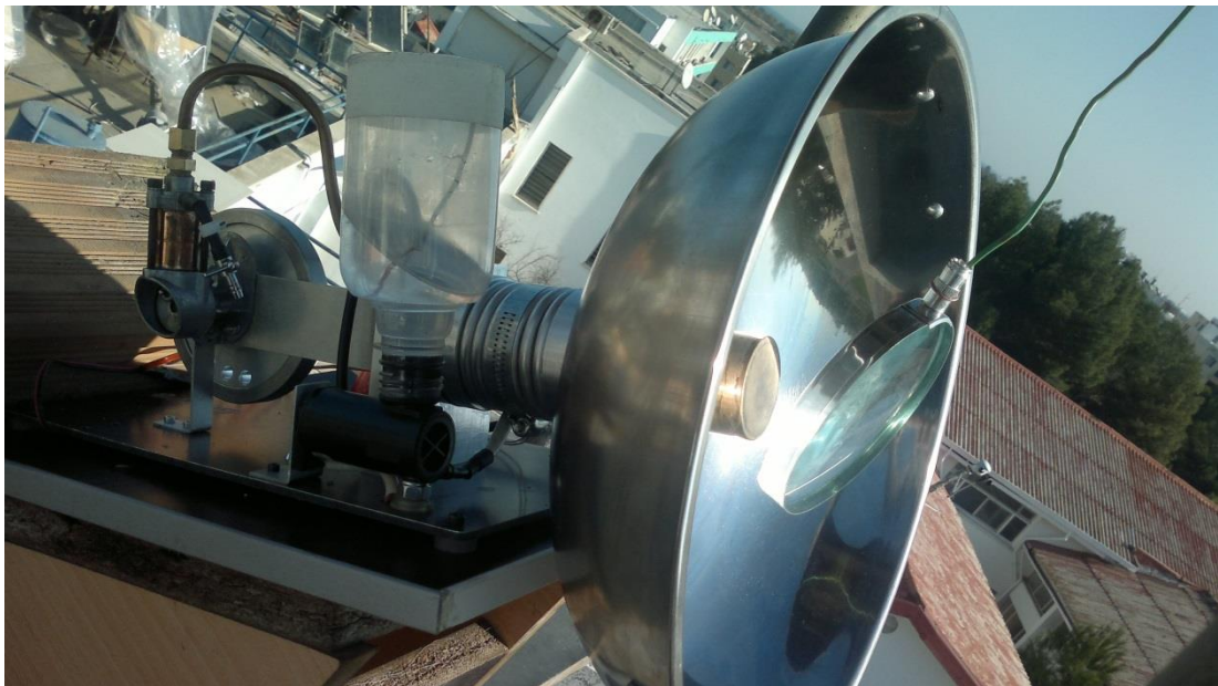
Figure 4.8 Prototype Stirling engine tested by solar radiation
