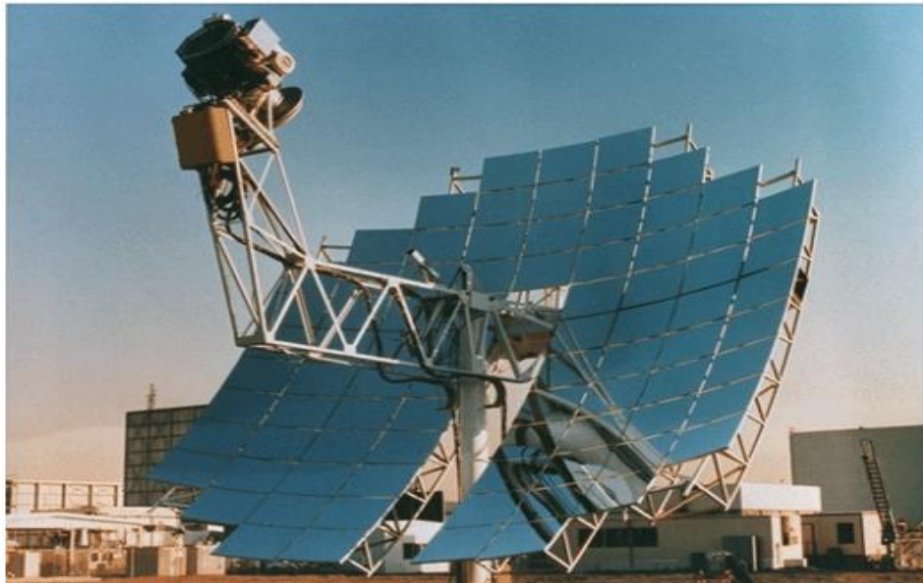
Figure 2.5. Solar Stirling engine system by McDonnell Douglas (1985) [8]
