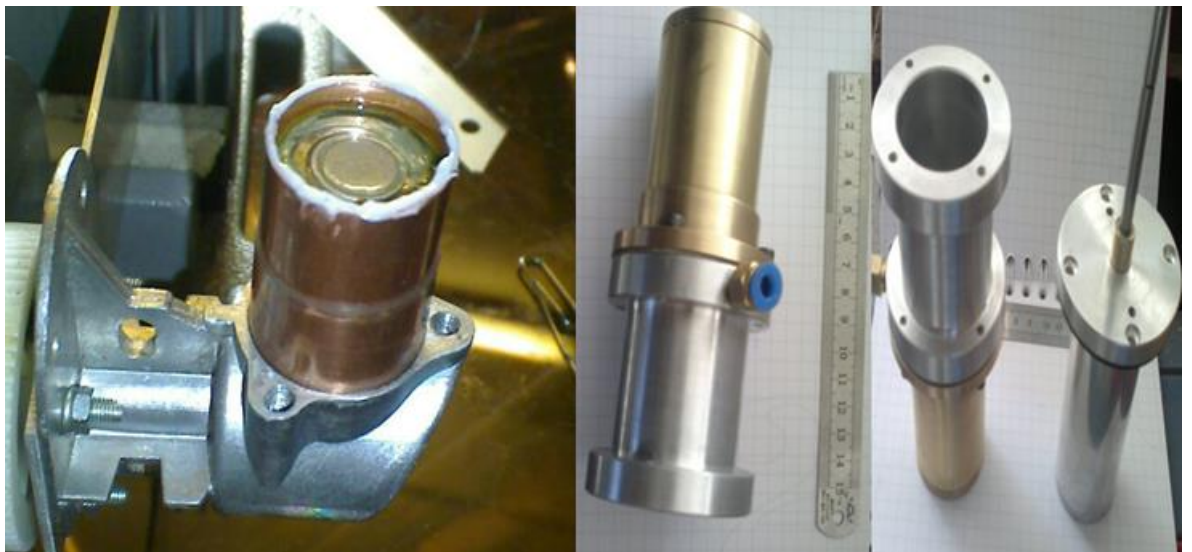
Figure 3.5. Cold side and heat side exchangers of designed prototype
