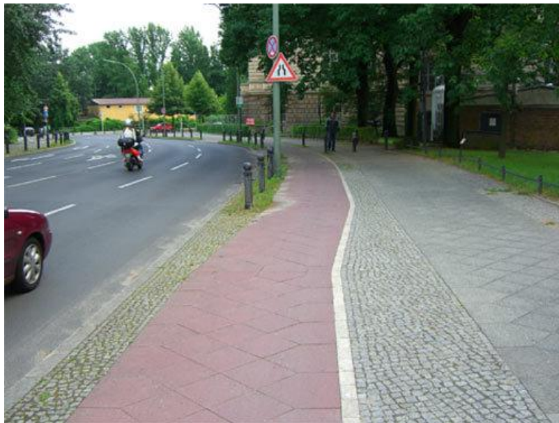
Figure 3.3 A separated bike lane with sidewalk in Berlin, Germany
