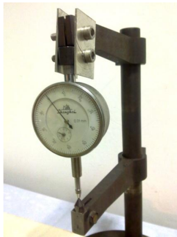
Figure 2.23 Point micrometer adapted for assessment of sheet thickness at h_f
