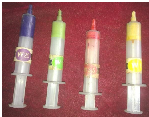
Figure 2.13 Diamond paste of different abrasive particle size, used for polishing of tool tip
