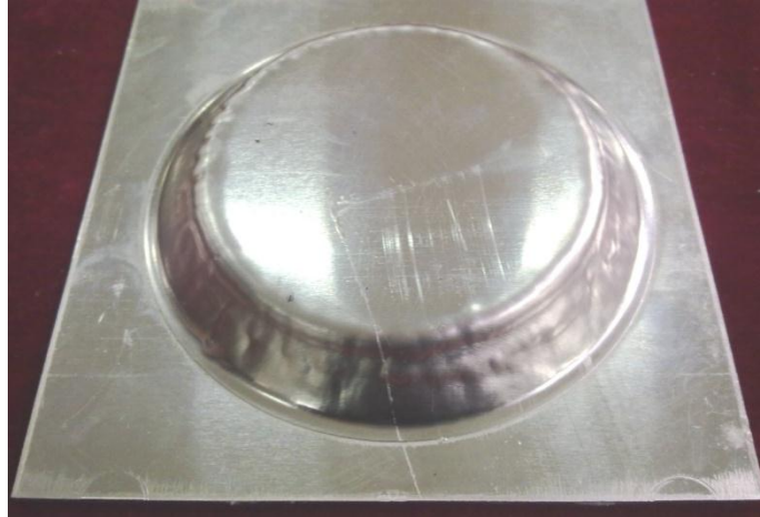
Figure 2.8 The effect of excessive frictional stress at the back side of specimen
