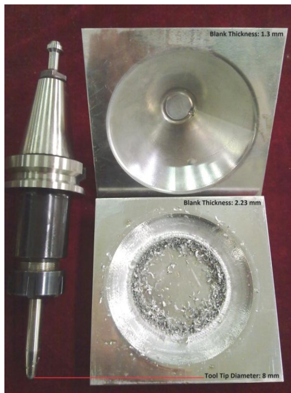
Figure 2.4 Two parts formed by identical process parameters and different thickness. This phenomenon can be realized due to accumulation of different causes, which can be explained with the aid of the model proposed by Silva et al. (2008), for the mechanism of ISF (Figure 2.5).
