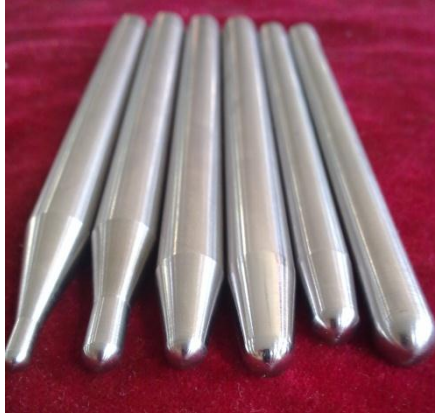
Figure 2.11 Forming tools in six various tip size
