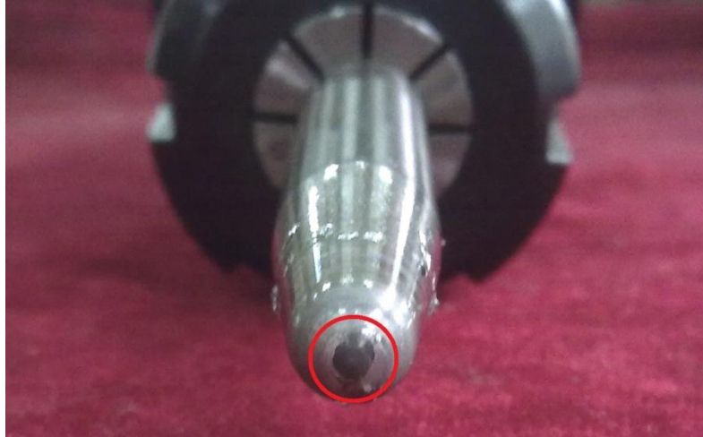
Figure 2.7 Adherence of sheet material to tool tip
