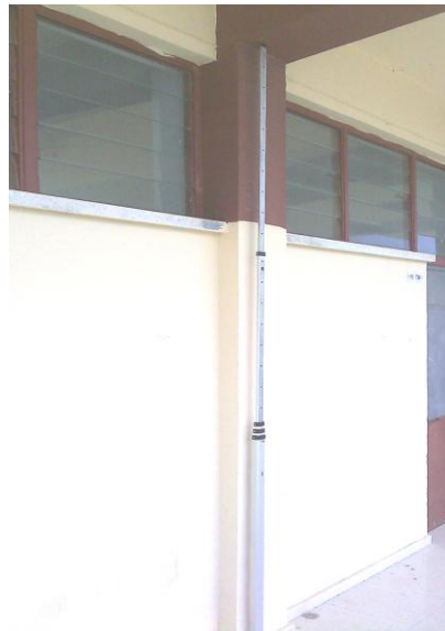
Figure 4.1: Showing expandable staff; measuring height of column
