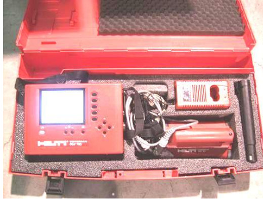
Figure 4.21: Ferro scan device
