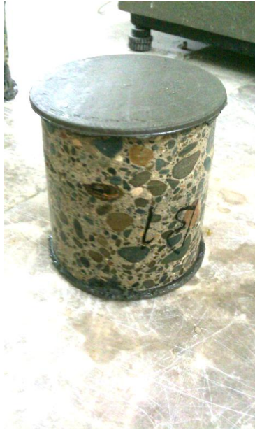
Figure 4.25: Showing capped concrete core sample
