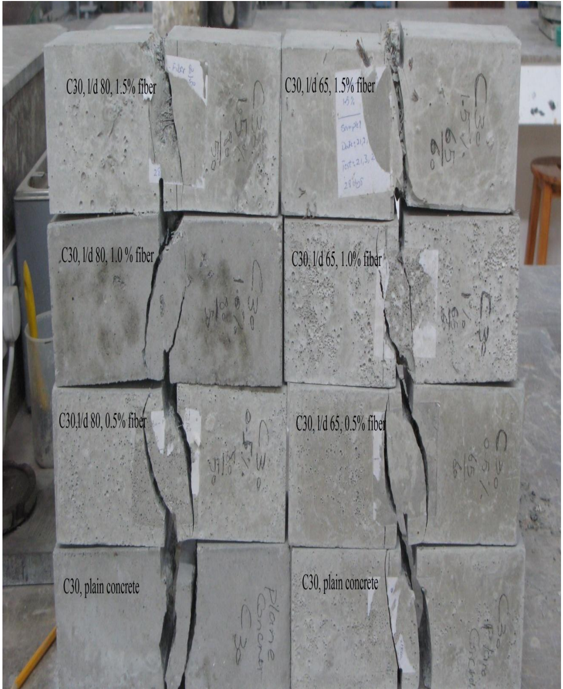
Figure 73: C30 with two different volume fraction of fibers
