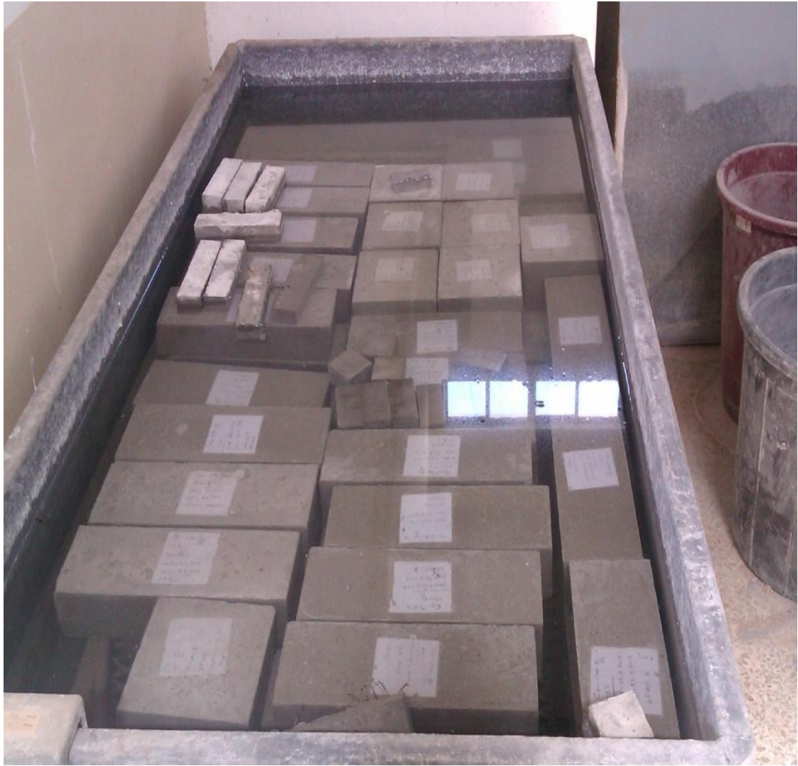
Figure 28: Water curing tank
