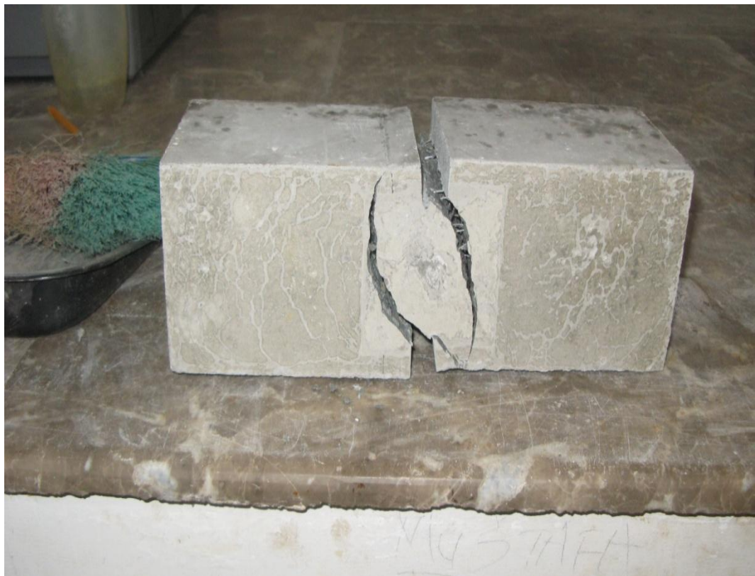
Figure 71: SFRC after cracking
