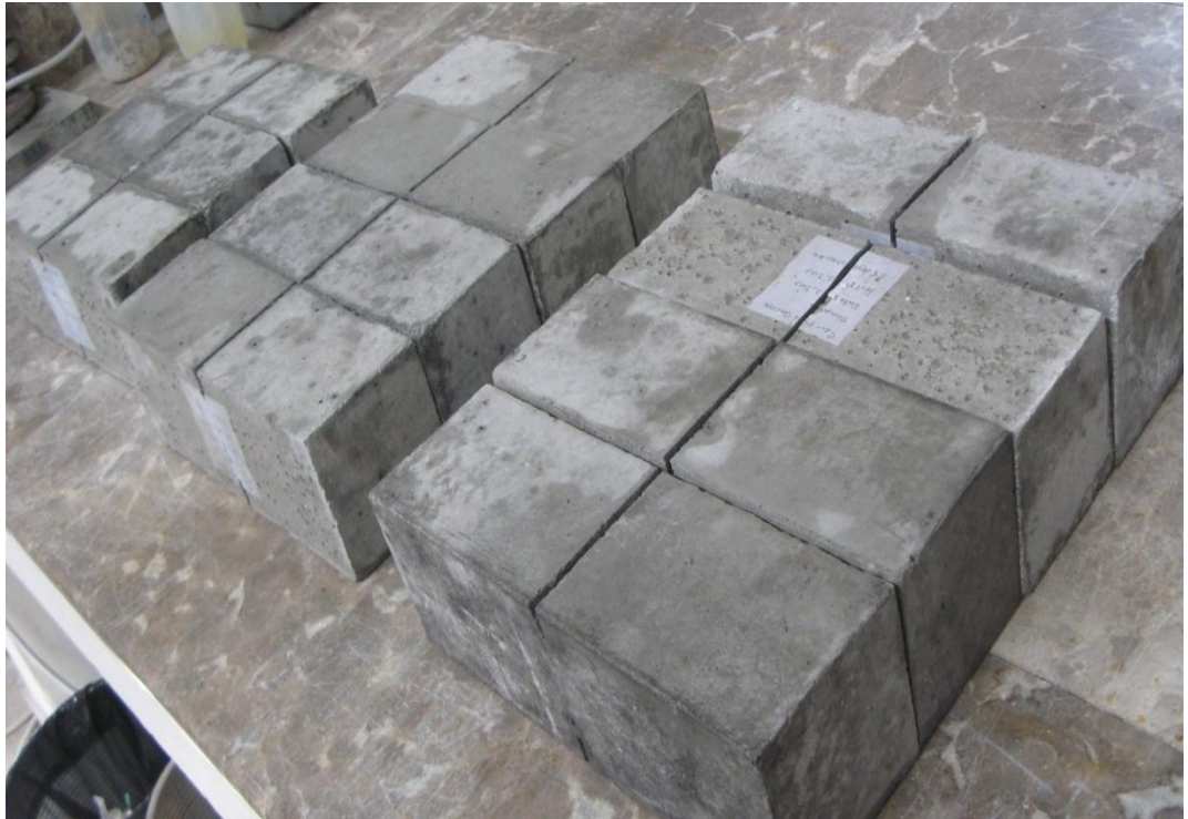
Figure 37: prepared samples for shear test
