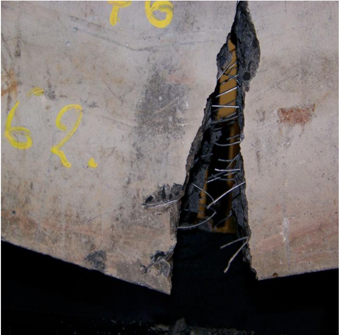
Figure 14: behavior of FRC after shear loading
