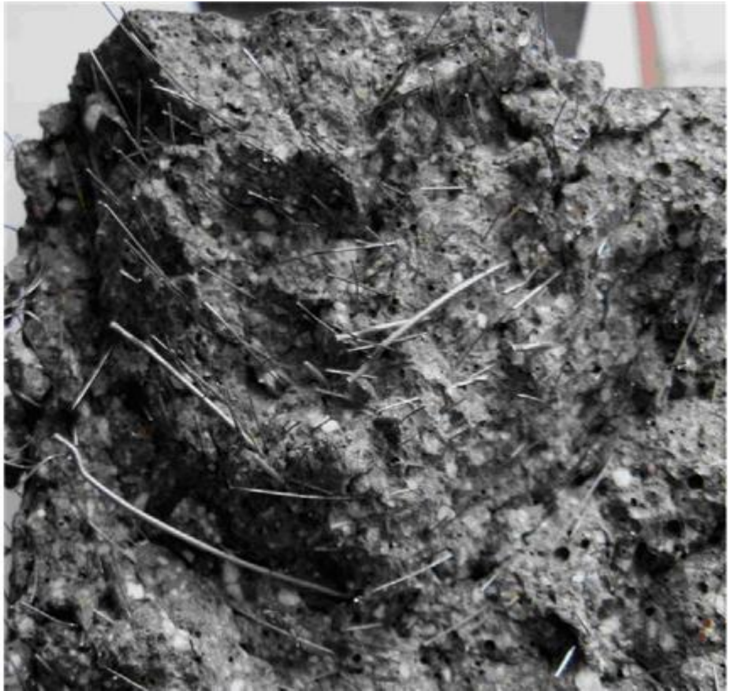
Figure 10: mortar mixed by fibers (Jsce.or.jp, 2013)
