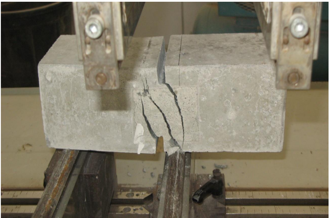
Figure 67: Fibers prevent separation
