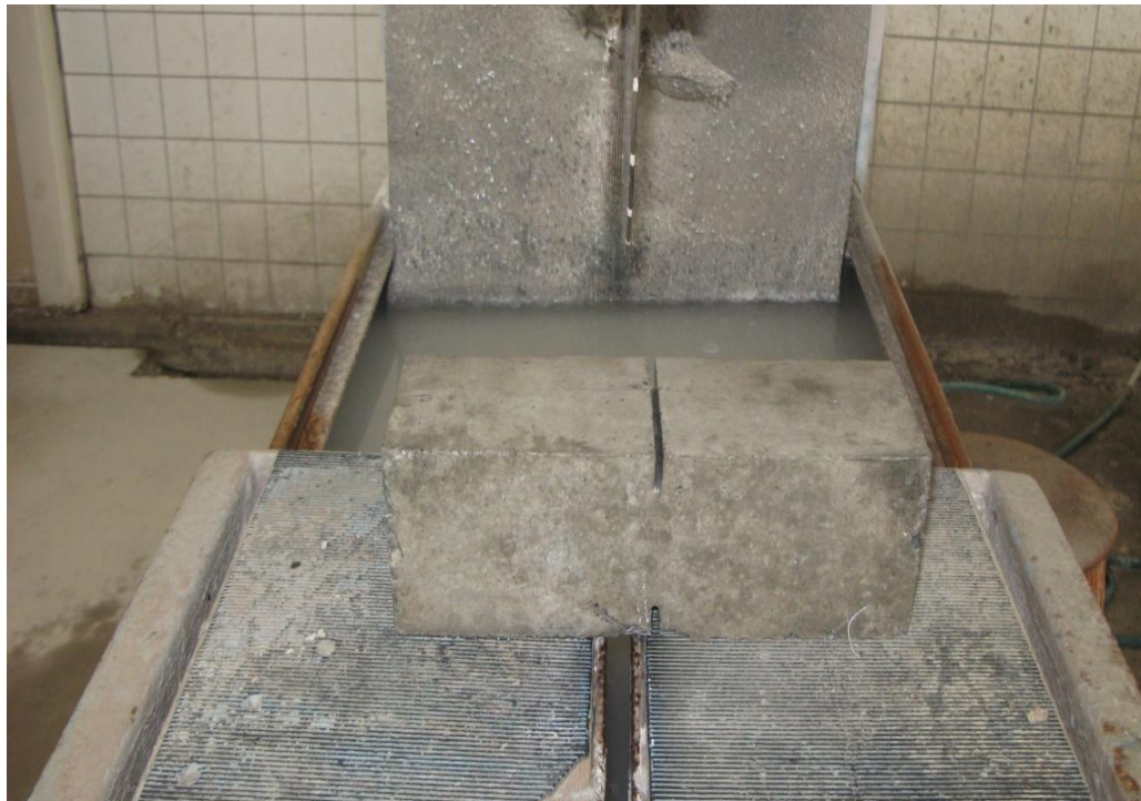
Figure 36: cutting sample for shear test
