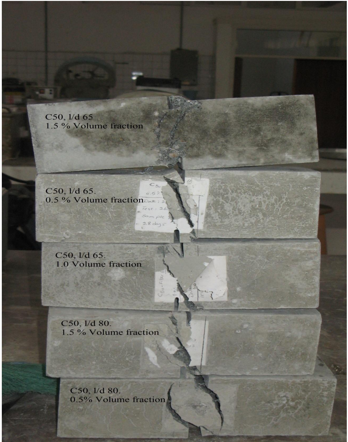
Figure 72: Effectiveness of using different amounts of steel fiber
