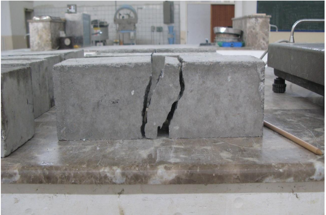
Figure 64: Sample after shear failure
