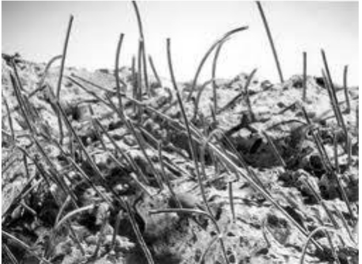
Figure 18: Orientation of fiber in concrete and mortar (Jsce.or.pi, 2013)
