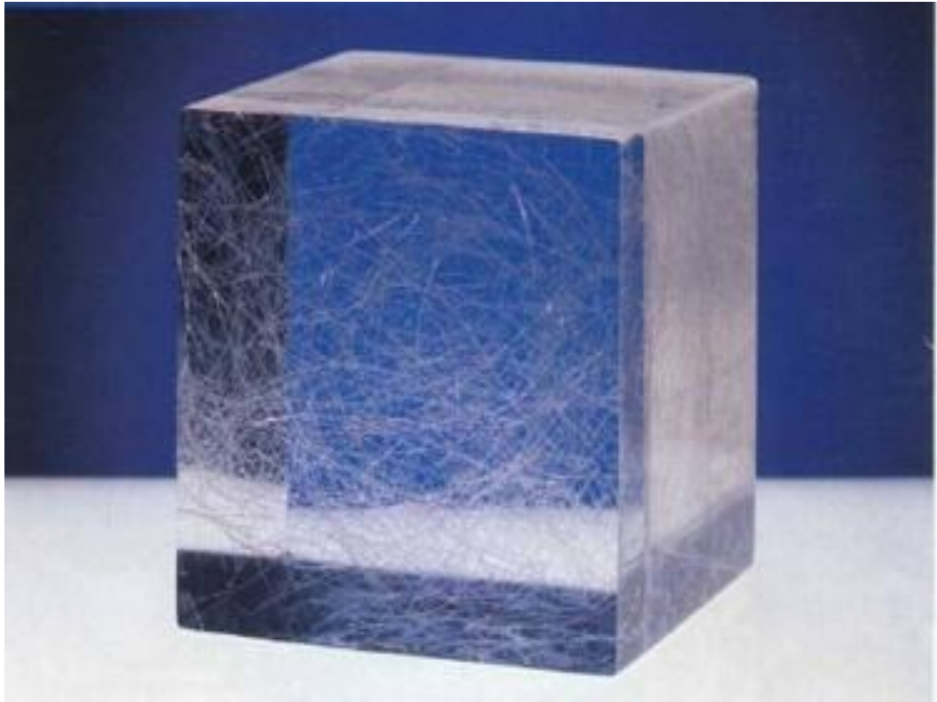
Figure 6: Orientation of glass fibers (construction.sunroc.com, 2013)
