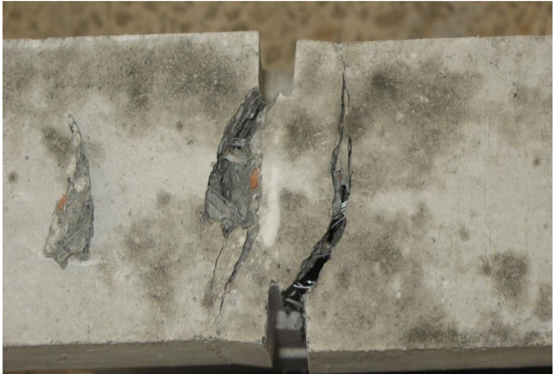
Figure 70: Affected sample by steel fiber
