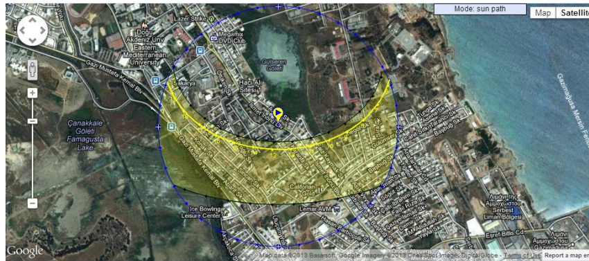
Figure 3.9: Sun Path Diagram for the Case Study Shown by Yellow Color (Illustration taken from URL: www.sunearthtools.com/dp/tools/pos_sun/php )
