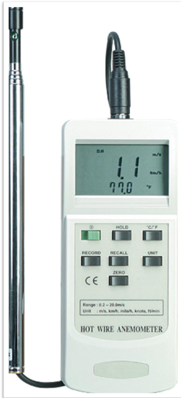
Figure 3.6: Hot Wire Anemometer [58].
