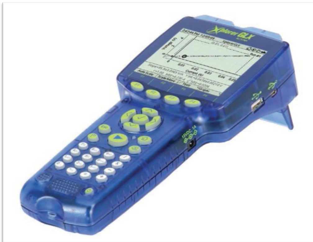
Figure 3.9: Xplorer GLX Pasco temperature measurement device [63].
