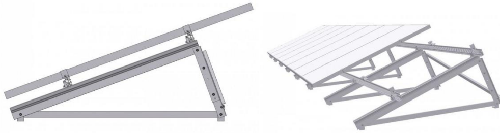
Figure 4.18: Side View and Perspective Drawing of Profile Carriers for Flat Roofs
