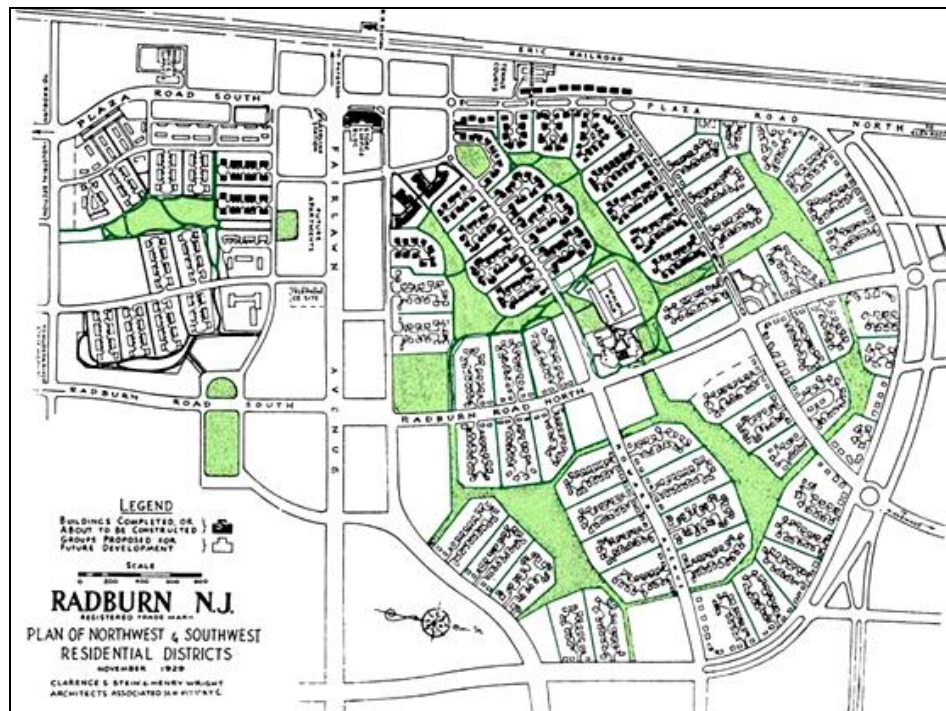
Figure 2.5. The “Radburn Idea.” Neighbourhood Layout with large “superblocks” designed to separate automobiles from pedestrians. (Source: Schaffer 1992)
