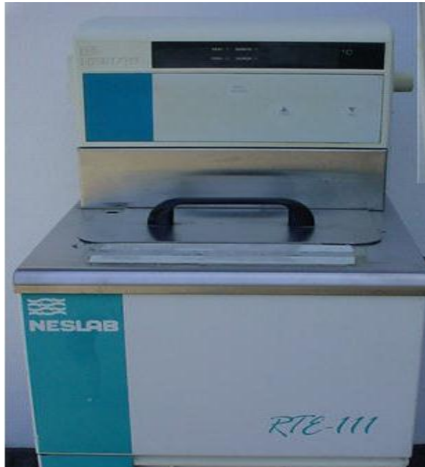
Figure 13. Constant temperature bath used for the experiment
