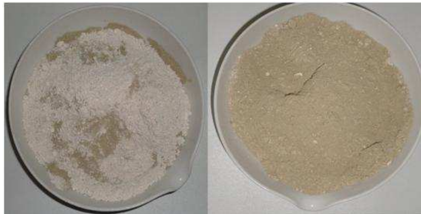
Figure 3.9: Mixture of Posidonia oceanica ash and soil for Atterberg limit analysis
