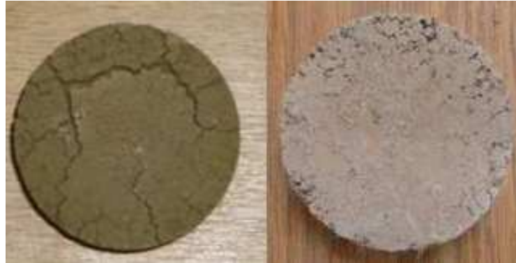
Figure 4.6: Crack pattern on unreinforced and reinforced specimen
