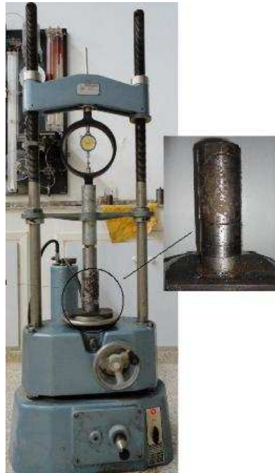
Figure 3.3: CBR equipment and the mold used for static compaction
