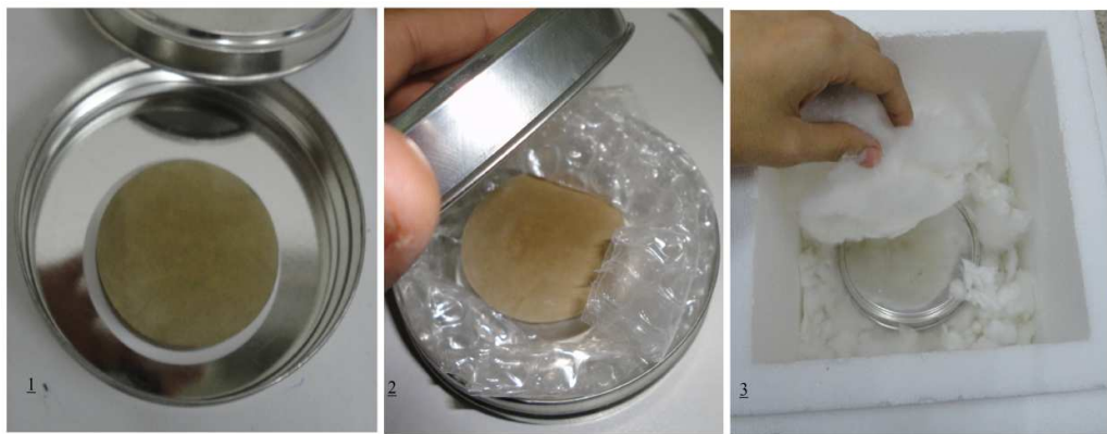
Figure 3.7: Packing of soil samples for suction measurement with filter paper method
