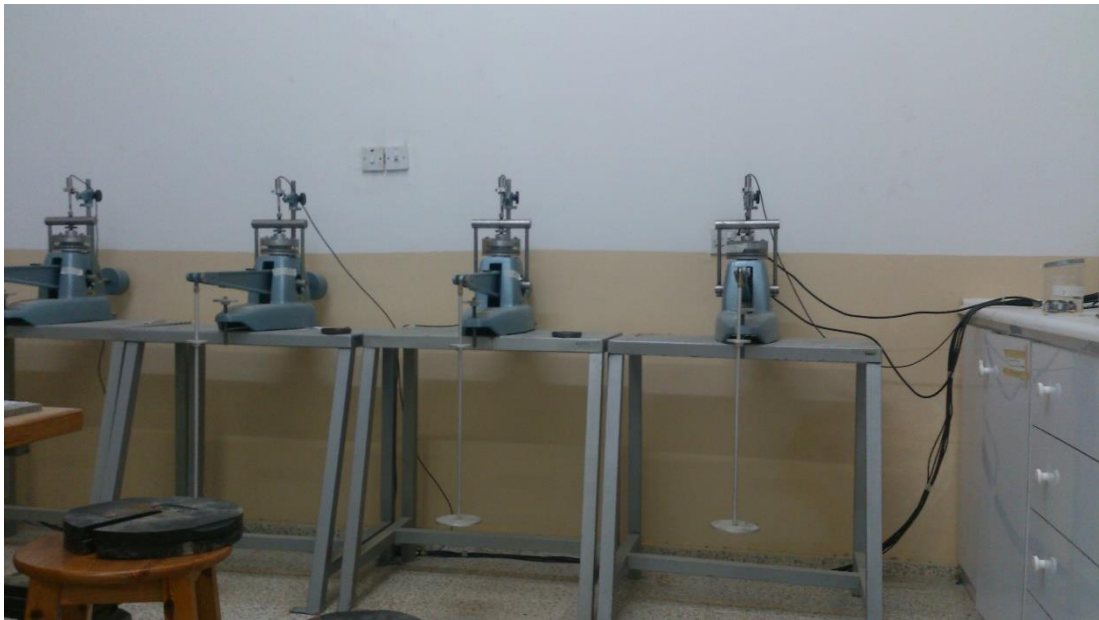
Figure 3.3: One-dimensional swell-consolidation tests run with transducers.
