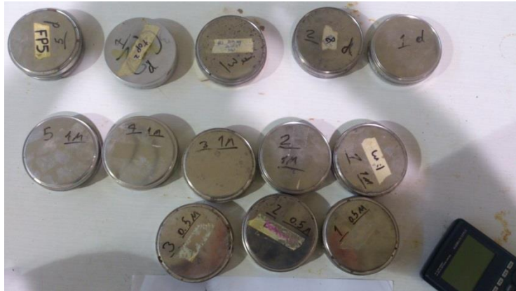
Figure 3.6: Compacted and saturated samples sealed in moisture containers.
