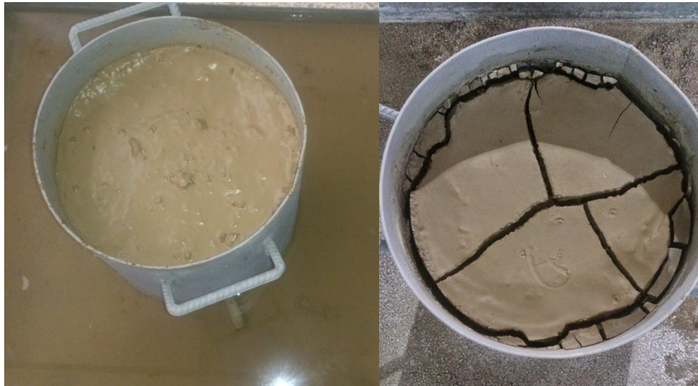
Figure 3.9: (a) saturated soil, (b) Desiccating soil with surface cracks.
