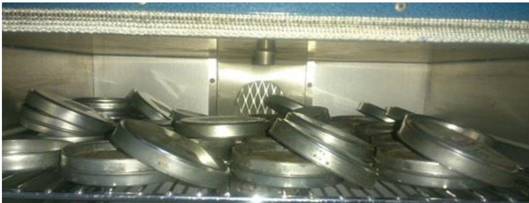
Figure 3.7: Desiccation of saturated samples in the oven at 40° C.
