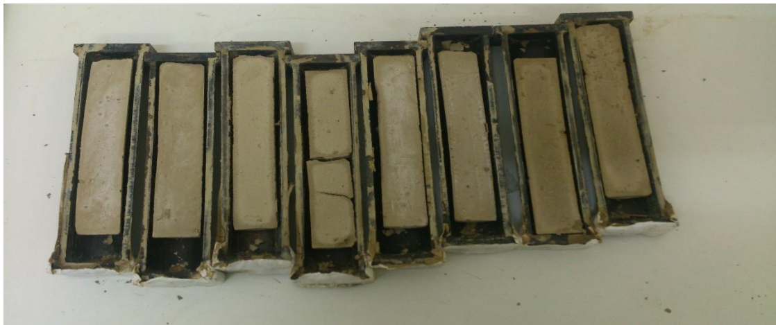
Figure 3.1: Linear shrinkage test molds and dried samples of varying pore-water chemistry.
