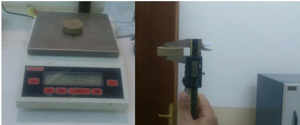
Figure 3.2: Volumetric shrinkage test: Measurements of (a) mass, (b) dimensions of drying specimens.
