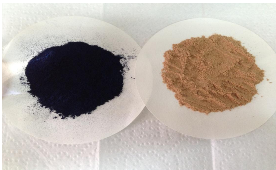
Figure 2.3: Palm seeds before and after MB adsorption.
