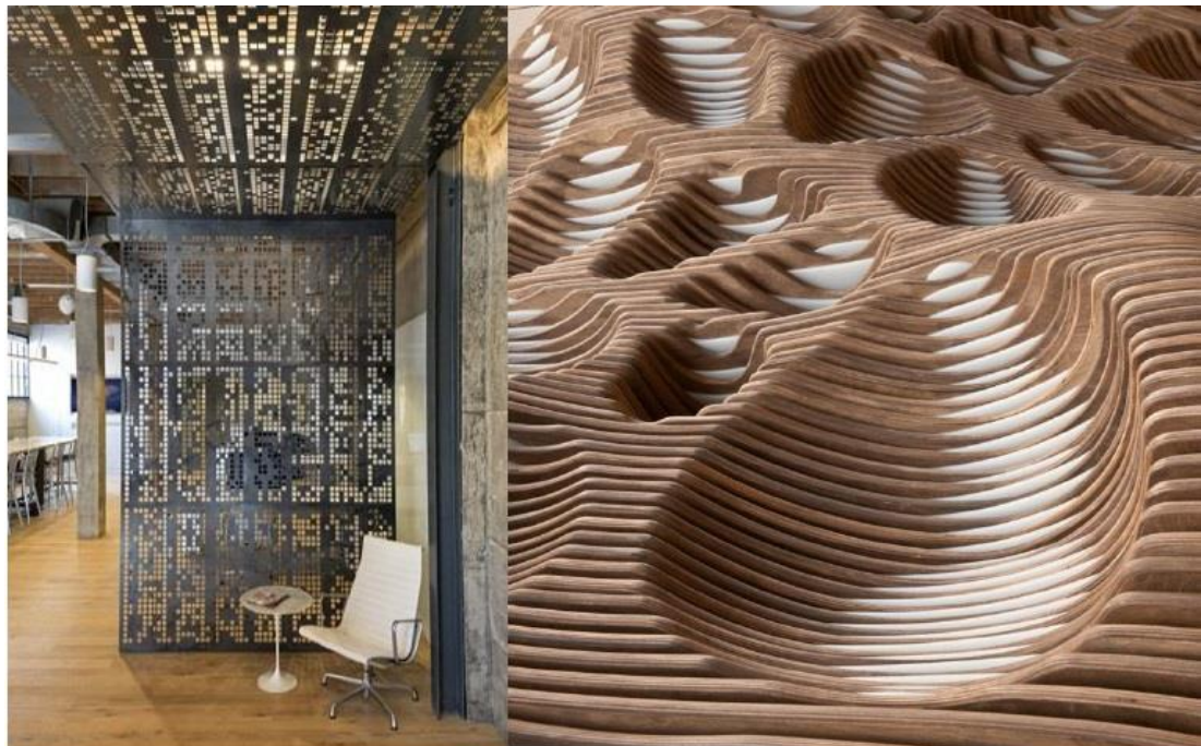
Figure 18: Left: CNC cutting laser panel design, Right: CNC router parametric design, Washington University School of Architecture class project Source: (Evolo, 2012)
