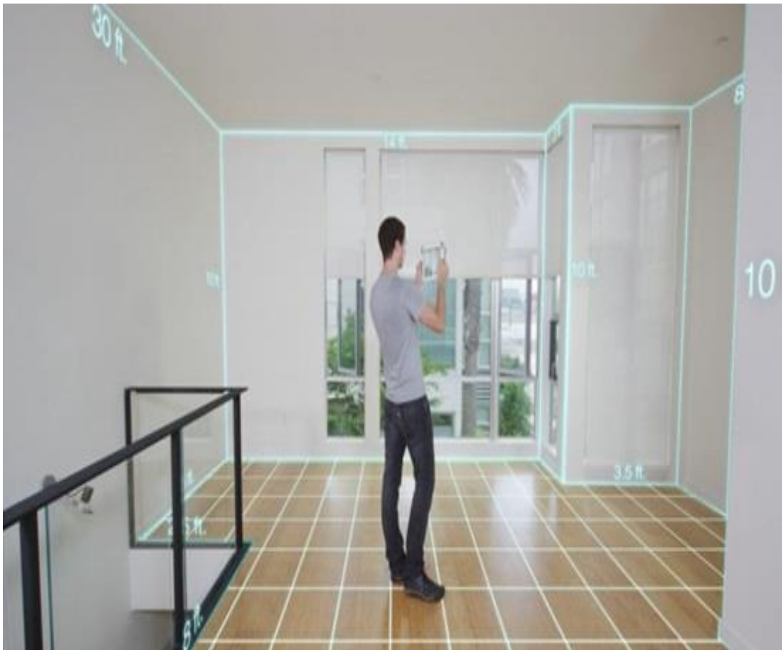
Figure 19: Structure Sensor scan a whole room and provide measurements with an iPad Apple application Source: (Hoops, 2013).
