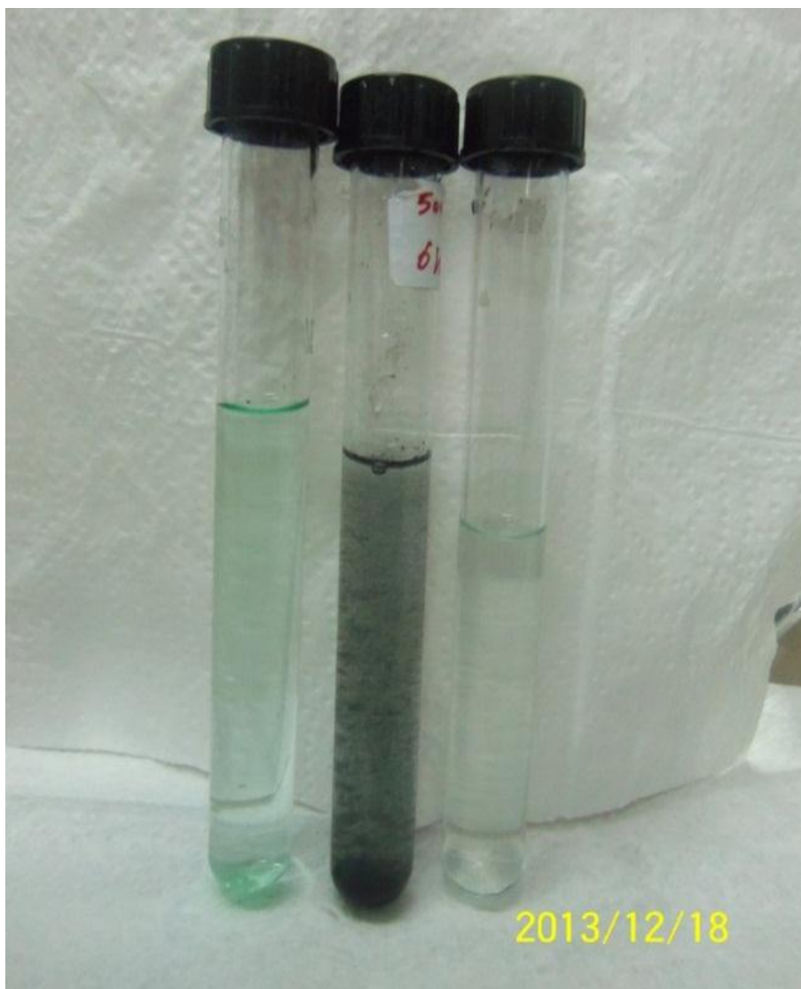
Figure 3.2: Nickel 2+ solution before addition of adsorbent (left test tube), with adsorbent in the (middle), and after the removal of the adsorbent (right). Images clearly shows the almost complete disappearance of the blue/greenish hue due to Ni 2+ cation.
