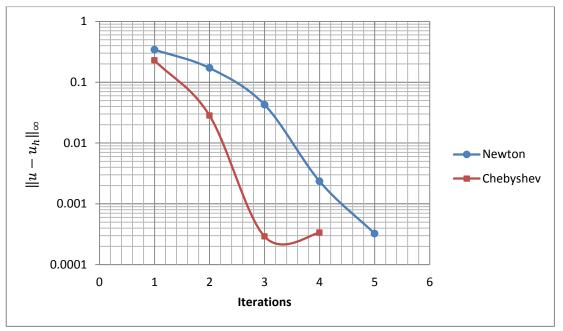
Figure 4.2: Comparison of the Convergency of (NM) and (CM) Using 5-Point Scheme for h=1/4.
