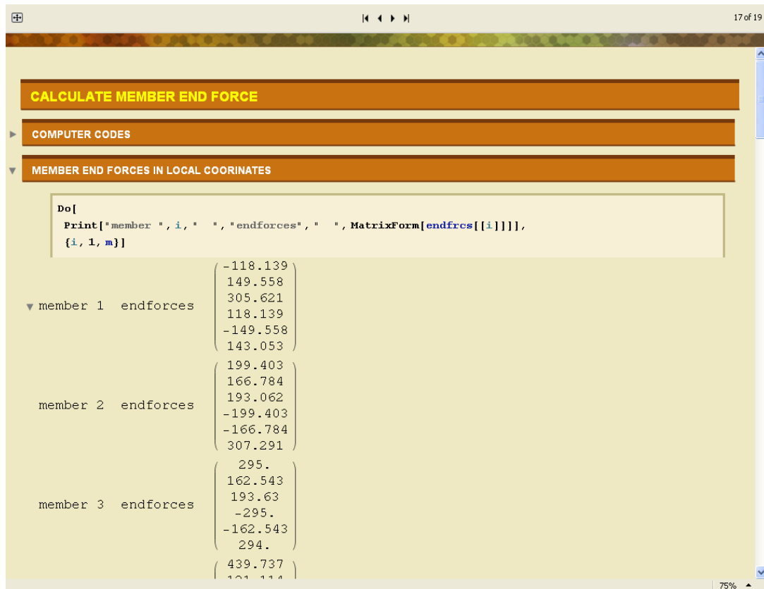
Figure 26: Reporting Results Phase, section 2, member end forces of member 1,2,3 in local coordinate
