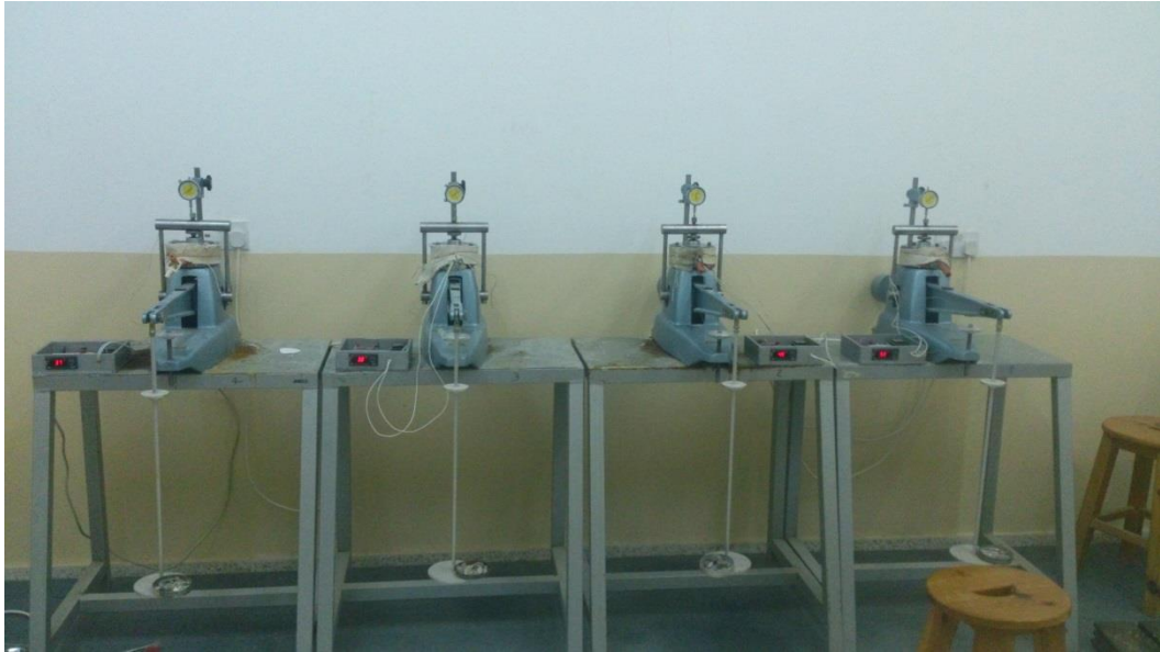
Figure 3.5: Consolidation under different temperatures
