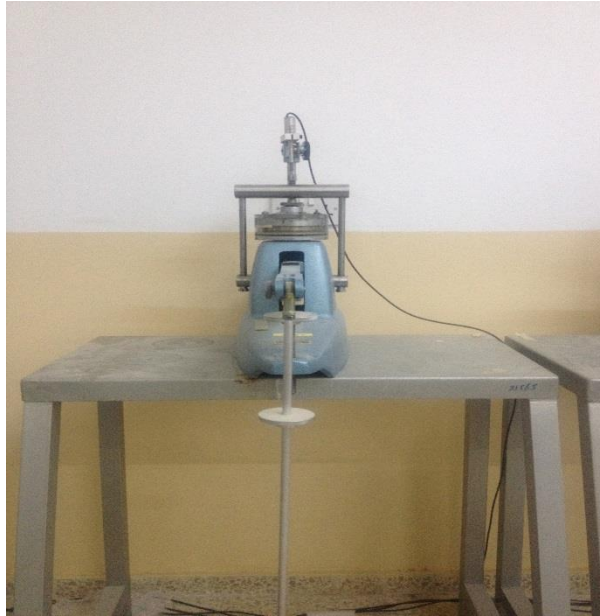
Figure 3.3: Consolidometer used in one-dimensional swell test.
