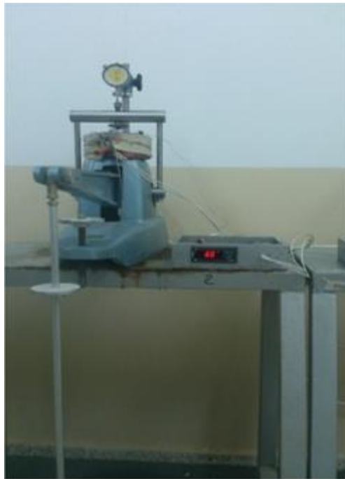
Figure 3.9: One-dimensional consolidation test under different temperatures
