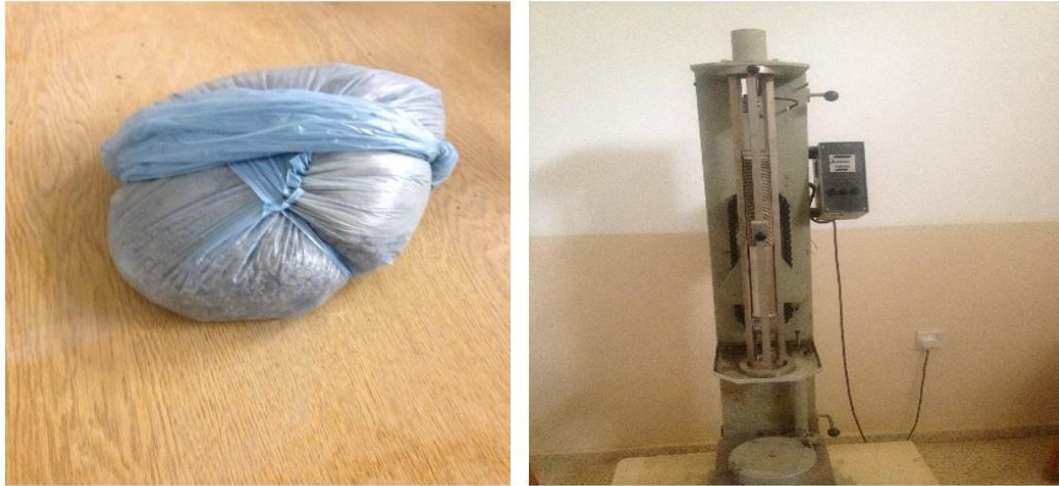
Figure 3.2: (a) Wet soil prepared and mellowed in nylon bag, (b) Dynamic compactor
