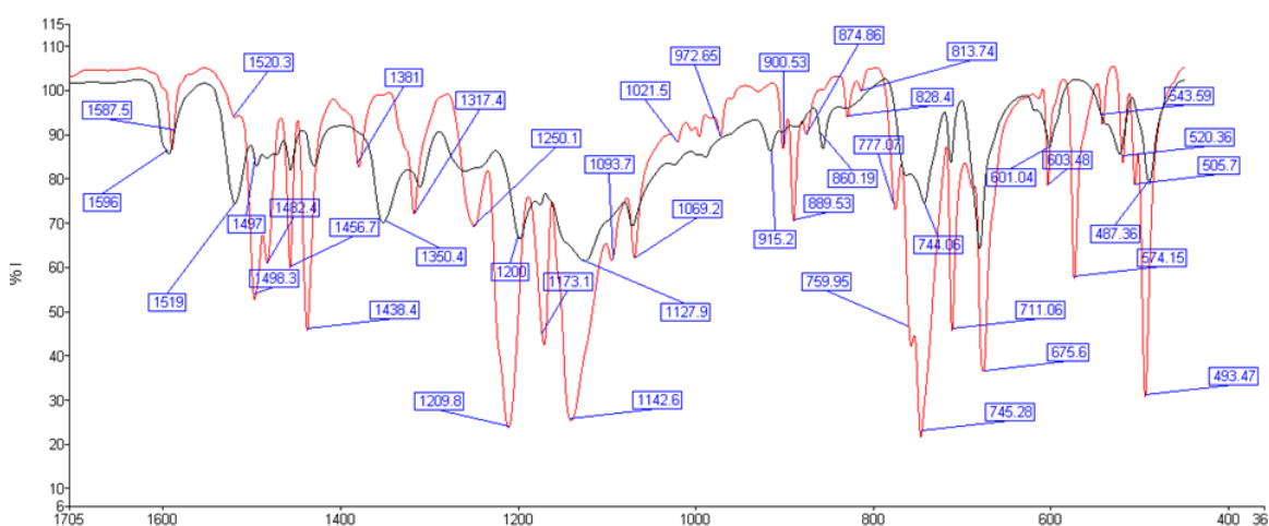
Figure 13: Overlapping Infrared Spectra Between 1700 and 400\text{ cm}^{-1} of Dithizone (Red line) and Dithizone-Cd Complex (Black line)
