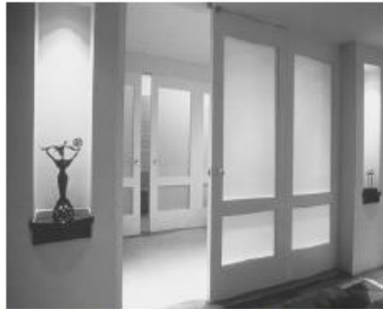
Figure 3.3 An example of concentrated downward distribution.
