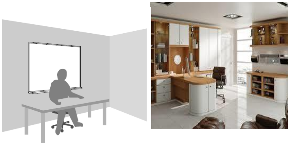
Figure 3.21: Arranging furniture such that the window is behind the back of the user (Daylight in Buildings)
