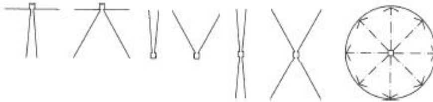
Figure 3.1 The seven directions and distributions of light.
