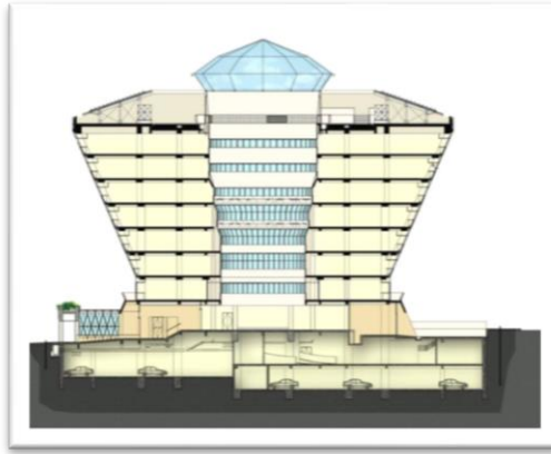
Figure 4.17: 25° Cross Section (Façade Tilt Angle) (www.mesym.com)
