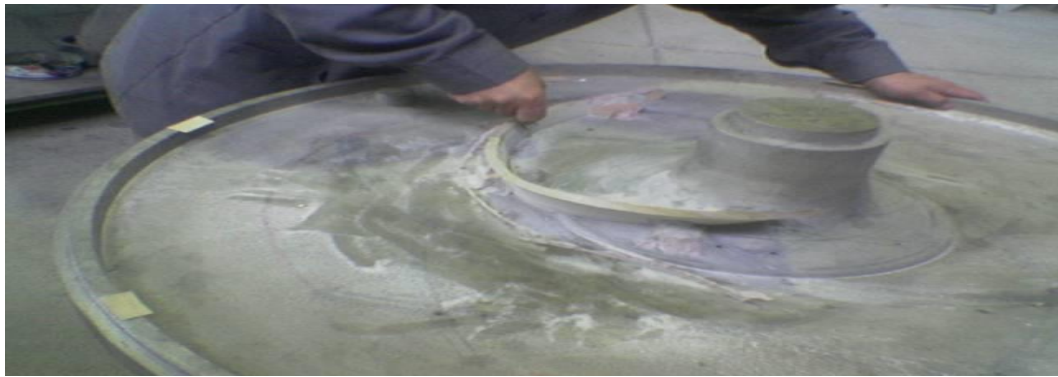
Figure 34: Wooden blade is prepared to making core box
