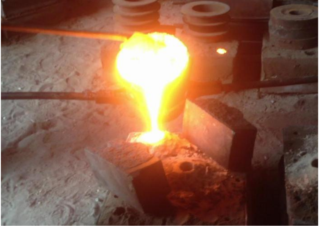
Figure 47: filling the die with melted cast iron
