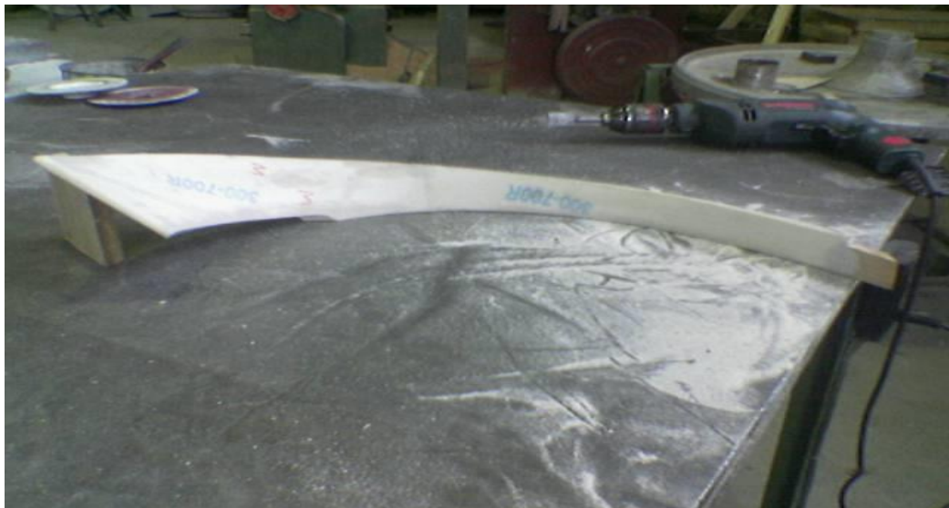
Figure 33: conventional core box making
