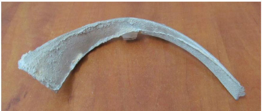
Figure 40: This Prototyped Blade will be used to Produce Aluminum Blade which are used Inside of Core Box
