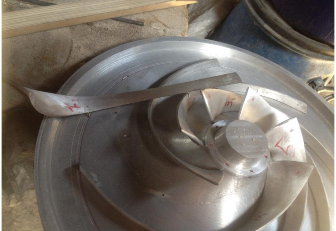
Figure 40: The Blades Prepared and Joined to Main Core Box via small pins which Located in down side of impeller shroud
