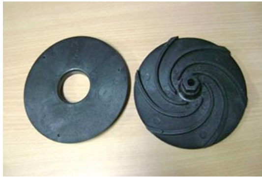
Figure 23: This impeller can use as core box directly
