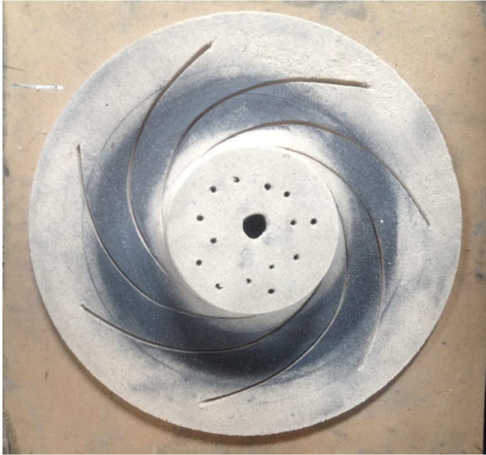
Figure 42: Prepared Sand Core via using Aluminum blades
