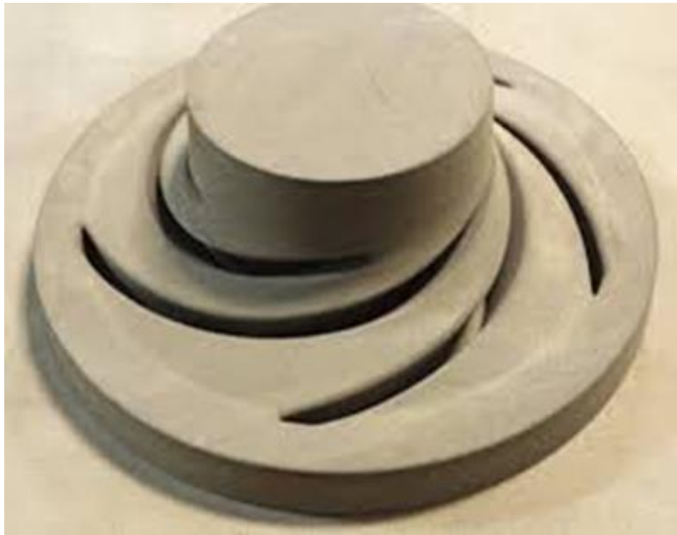
Figure 26: Produced core via using 2D impeller directly as a core box
