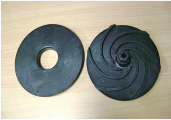
Figure 19: 2D blade open impeller
