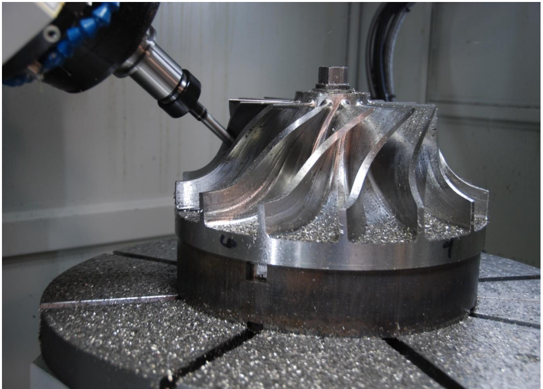
Figure 16: Directly machining of impeller via CNC machine
