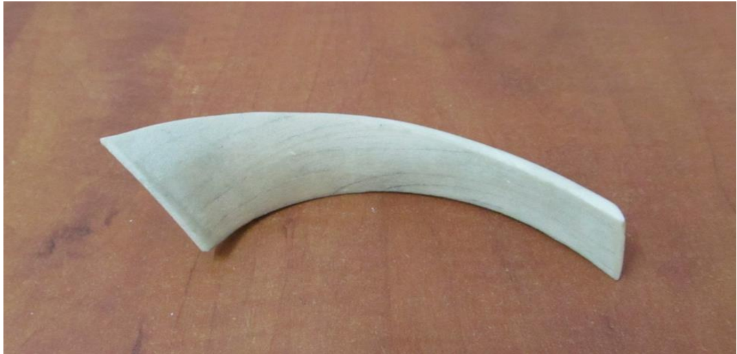
Figure 39: Blade of Prototyped Impeller Via 3D Printing Machine
