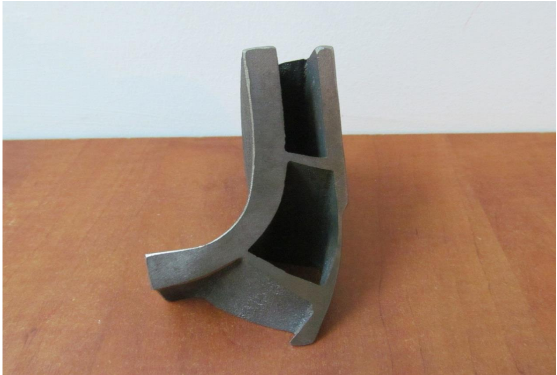
Figure 36: Cut Impeller Ready to Scan
