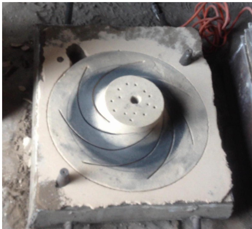
Figure 44: Sand Core is Accommodate on Top of Down part
