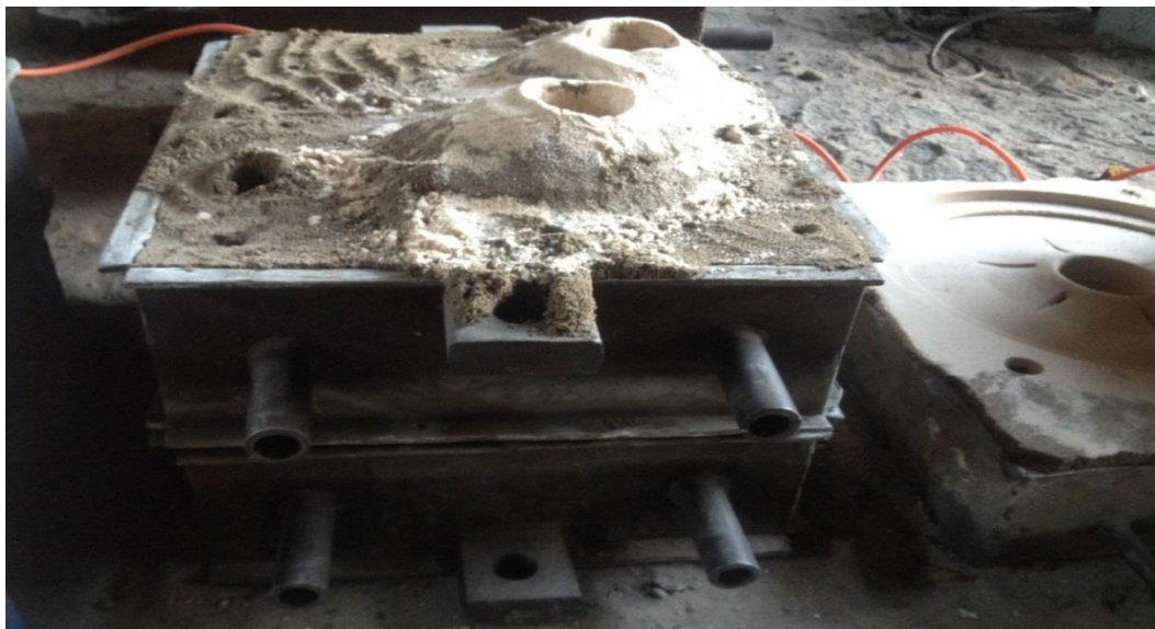
Figure 46: Montaged Die and it is Ready to Pour the molten material.
