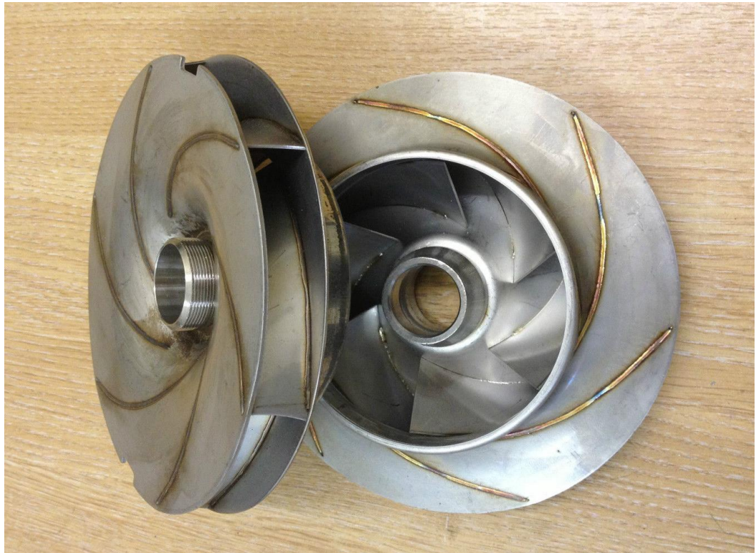
Figure 17: Impeller manufactured via welding procedure
