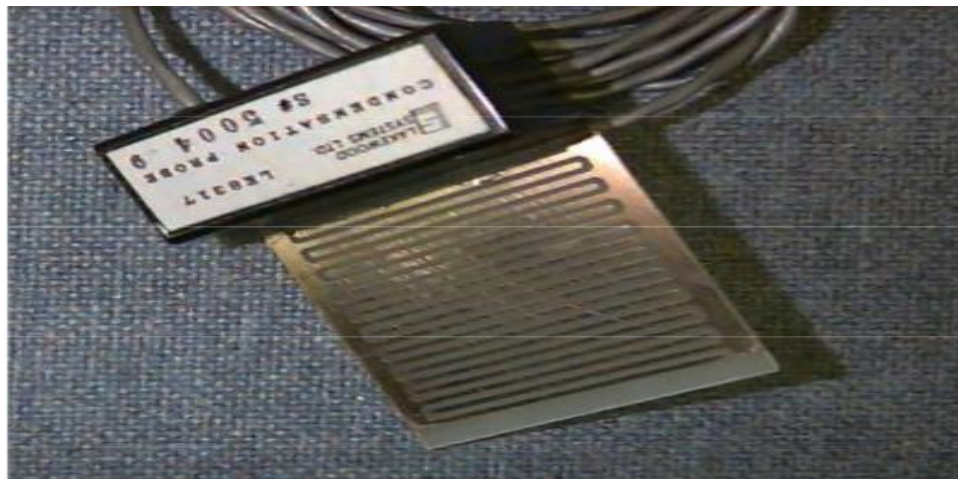
a) Printed circuit condensation moisture sensor
