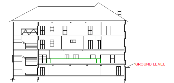
SECTIONAL VIEW OF COLONIAL POST OFFICE NICOSIA SHOWING BASEMENT GROUND, FIRST AND SECOND FLOORS
