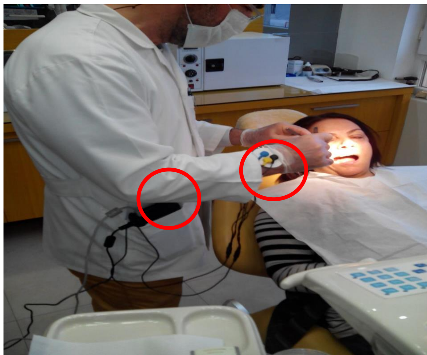
Figure 1. Placement of sEMG electrodes on hand/wrist ( musculi lumbricales manus ) and forearm ( extensor carpi radialis )
