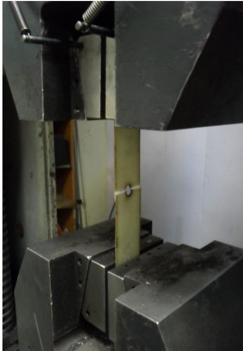
Figure 5.6: Fracture point after Laser machining
