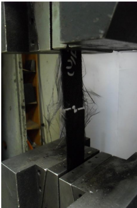
Figure 5.11: Fracture point after Water-jet machining
