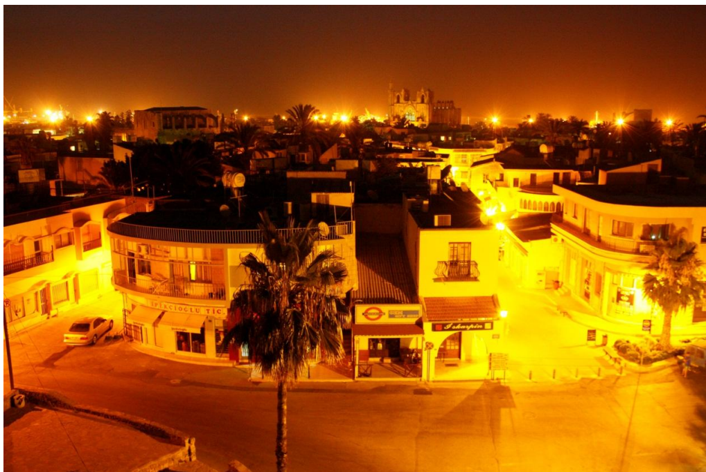
Figure 63: High pressure sodium lamps used for street lighting makes a saturated yellowish light with low level of CRI. (Photo by Author)
