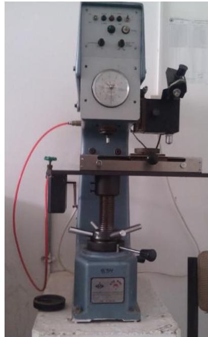
Figure 3.7: A View of Hardness Tester Machine used
