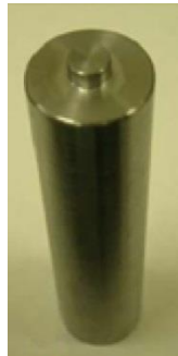
Figure 3.2: The Appropriate Tool used in Friction Stir Processing
