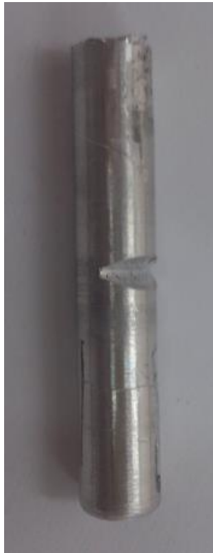
Figure 3.13: A Schematic of Grooved Pin
