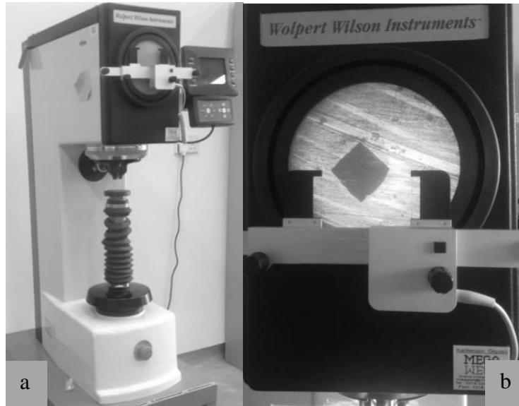
Figure 3.6: (a) Micro-hardness tester. (b) Optical and the measuring equipment.
