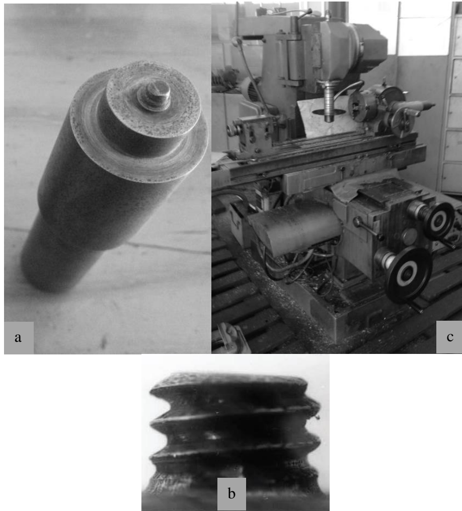
Figure 3.3: (a) Processing tool; (b) Threaded taper cylindrical pin; (c) Picture of milling machine used for friction stir processing.
