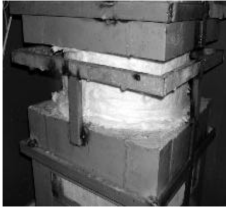
Figure 4.21: Wrapping isolator in fire insulation (Yilmaz et al., 2006).
