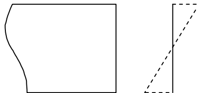
Figure 3.30: Strain distribution along all element sections
