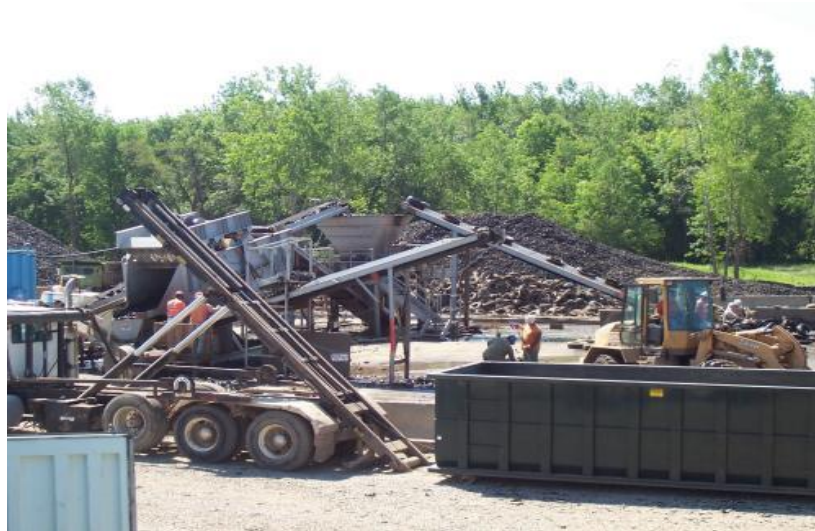
Figure 4: Tire shredding plant for pavement ( http://www.shredderhotline.com )
