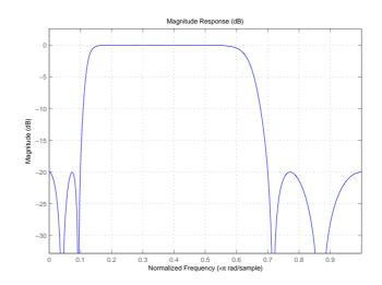
Figure 4.24. The magnitude response of the acoustic room.
