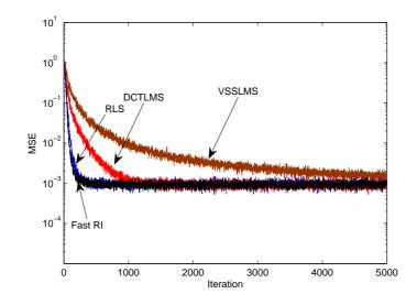
Figure 4.2. The ensemble MSE for the fast RI, RLS, VSSLMS and DCTLMS in AWGN.
