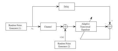
Figure 4.18. Block diagram of the adaptive equalization model.
