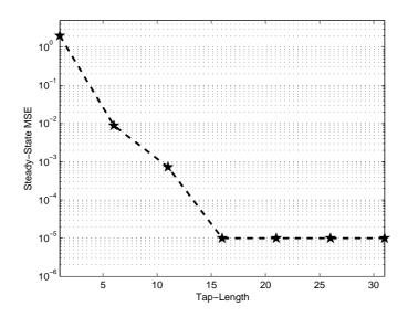
Figure 4.31. The curve of steady-state MSE with respect to the tap-length.
