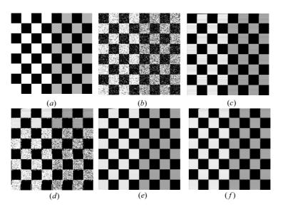
Figure 4.28. (a) Original image, (b) Image with noise, (c) Restored image using the 2D RI ( $\beta = 0.995$ ), (d) Restored image using the 2D RLS ( $\beta = 0.995$ ), (d) Restored image using the 2D RI algorithm ( $\beta = 0.9995$ ), and (f) Restored image using the 2D RLS algorithm ( $\beta = 0.9995$ ).
