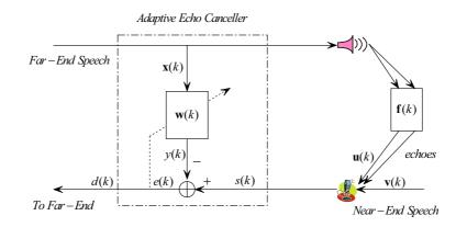
Figure 4.23. Block Diagram of a Typical Acoustic Echo Canceller.
