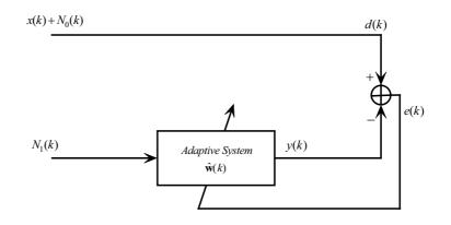
Figure 4.1. Block diagram of noise cancellation.
