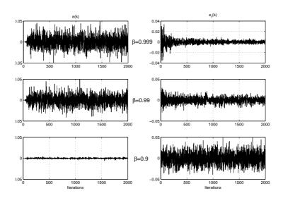
Figure 4.34. The leakage phenomenon of The RLS algorithm in time domain
