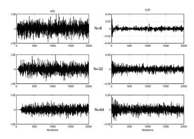
Figure 4.38. The leakage phenomenon of the RLS algorithm in time domain  $\beta=0.99 \text{ and different values of } N.$
