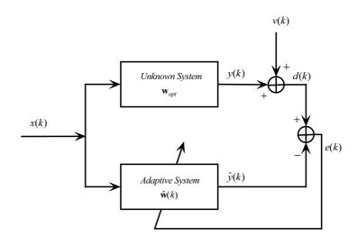
Figure 4.9. Block diagram of system identification.
