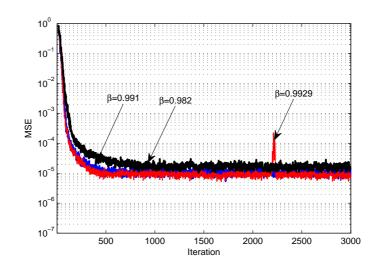
Figure 4.30. The ensemble MSE for the RI algorithm in AWGN with different values of  $\beta$ .
