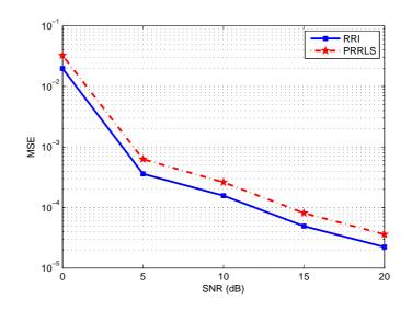
Figure 4.14. The ensemble MSE for the Robust RI and Robust RLS algorithms in AWIN for different SNR's ( $\epsilon = 0.01$ ,  $\kappa = 10000$ ).
