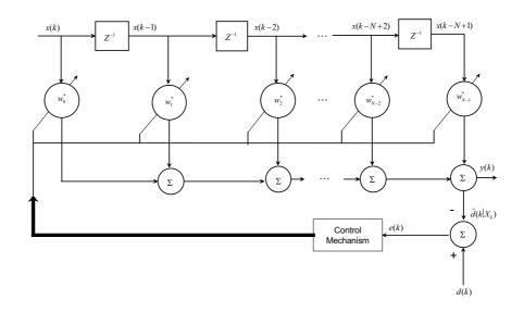
Figure 1.1. Structure of the adaptive transversal filter, [1].
