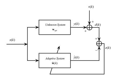
Figure 3.3. Block diagram of adaptive system identification.
