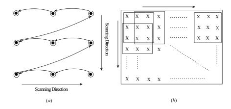
Figure 3.4. Rectangular Configuration of Data-Reusing in 2D.
