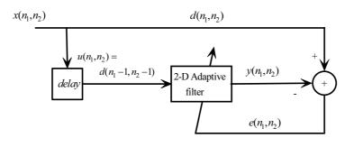
Figure 4.27. The block diagram of a 2D adaptive line enhancer.
