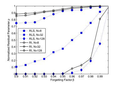
Figure 4.32. Normalized residual parameter  $\rho$  for different values of the forgetting factor  $\beta$  and the filter length N.
