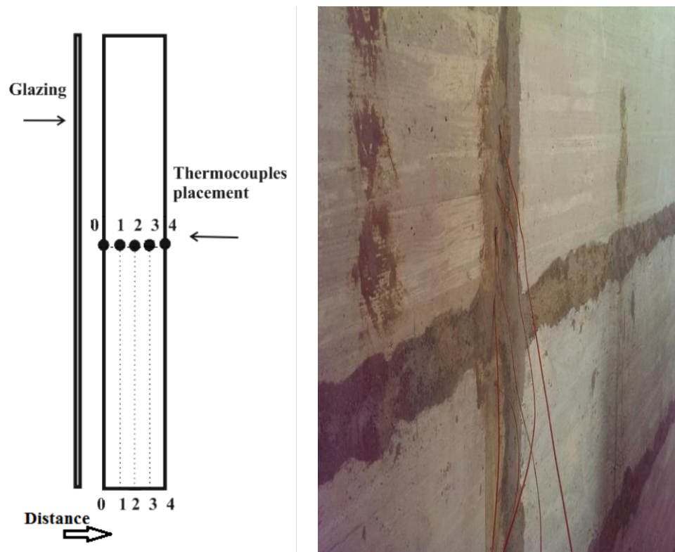
Figure 4.4. The cross section area of TSW and thermocouples placement.
