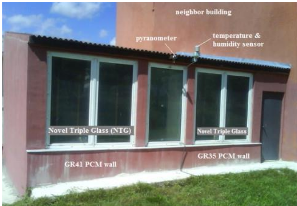
Figure 2.2. The test room used in experimental project of Ref. [8]
