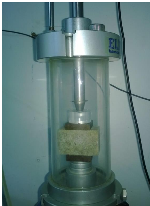
Figure 4.11. Cubic compressive strength test.
