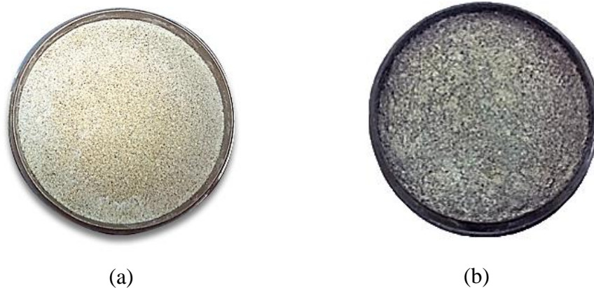
Figure 3.38. Sand bentonite cement sample after (a) first wetting –drying cycle, (b) fifth wetting–drying cycle.
