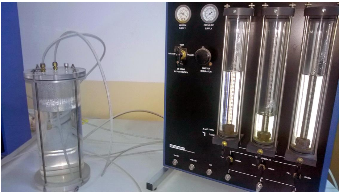
Figure 3.3. Tri-flex master control panel and de-airing tank system.
