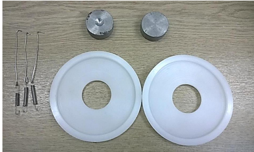
Figure 4.6. Top and bottom caps, metal discs and springs used for double punch test.
