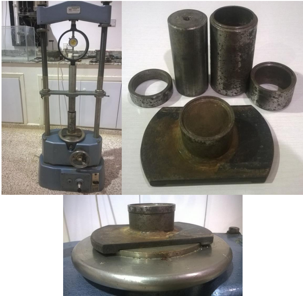
Figure 4.2. Static compaction (a) using CBR machine, (b) split tensile sample preparation mold, collar, hammer and bottom plate and (c) bottom plate modified for CBR.
